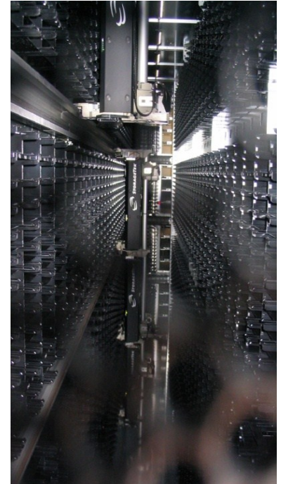
The StorageTek tape robot 100PB Capacity
