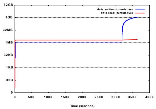
As can be seen, this file exists for the duration of the run, but it is in the final stages of the run that most of the data (over 1 GB) is written to the file. In our next figure we plot a histogram, showing the frequency of read and write requests versus request size, for the same "odb" file:
