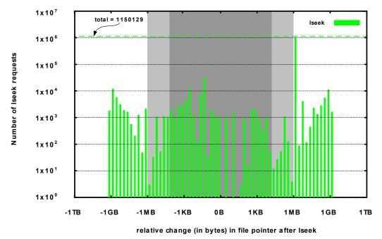
There are a substantial number of requests to lseek forward and backward by more than 1 GB. However, most of the requests (~1 million) are to lseek forward by more than 1 MB. The SFS is configured with a stripe size of 1 MB, so it should be clear that most of the lseek requests will force the file pointer to switch continuously between different file system stripes (OSTs).
