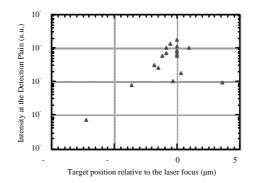
*Figure 2. Third harmonic intensity at the detector, as a function of target position relative to the laser focus*
