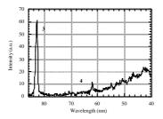
Figure 1. Typical lineout of the data taken with a laser intensity of  $2 \times 10^{18}$  Wcm<sup>-2</sup>, at an incidence angle of 28°, with the spectrometer in the specular reflection direction.
