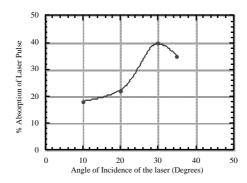
Figure 7. Percentage of the laser pulse absorbed by resonance absorption versus incidence angle of the laser, as measured by Borghesi et al. (16).
