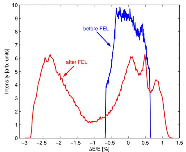
Figure 4: Results of GENESIS simulation: energy spread induced by the FEL interaction with 80 MW seed beam (data taken from Figs. 3(b) and (c)). Energies are shown relative to the mean input energy.
