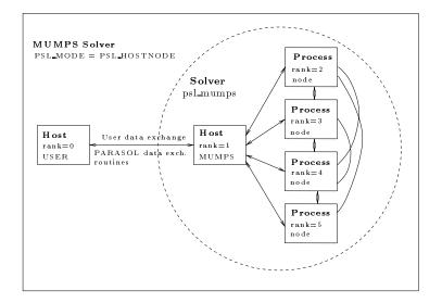
Figure 2.2: HOST\_NODE execution model for MUMPS
