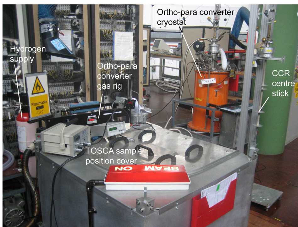
Figure 5.23: The TOSCA beamline with ortho-para hydrogen conversion rig and CCR centre stick before sample loading
