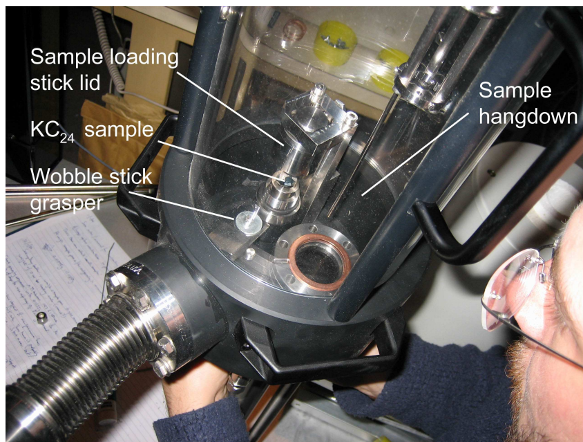
Figure 5.12: Unscrewing the IGA sample loading stick lid after purging, ready to load the sample holder onto the hangdown
