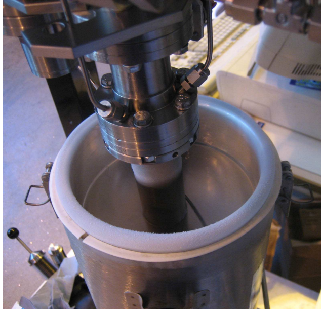
Figure 5.13: 77 K liquid nitrogen bath for IGA
