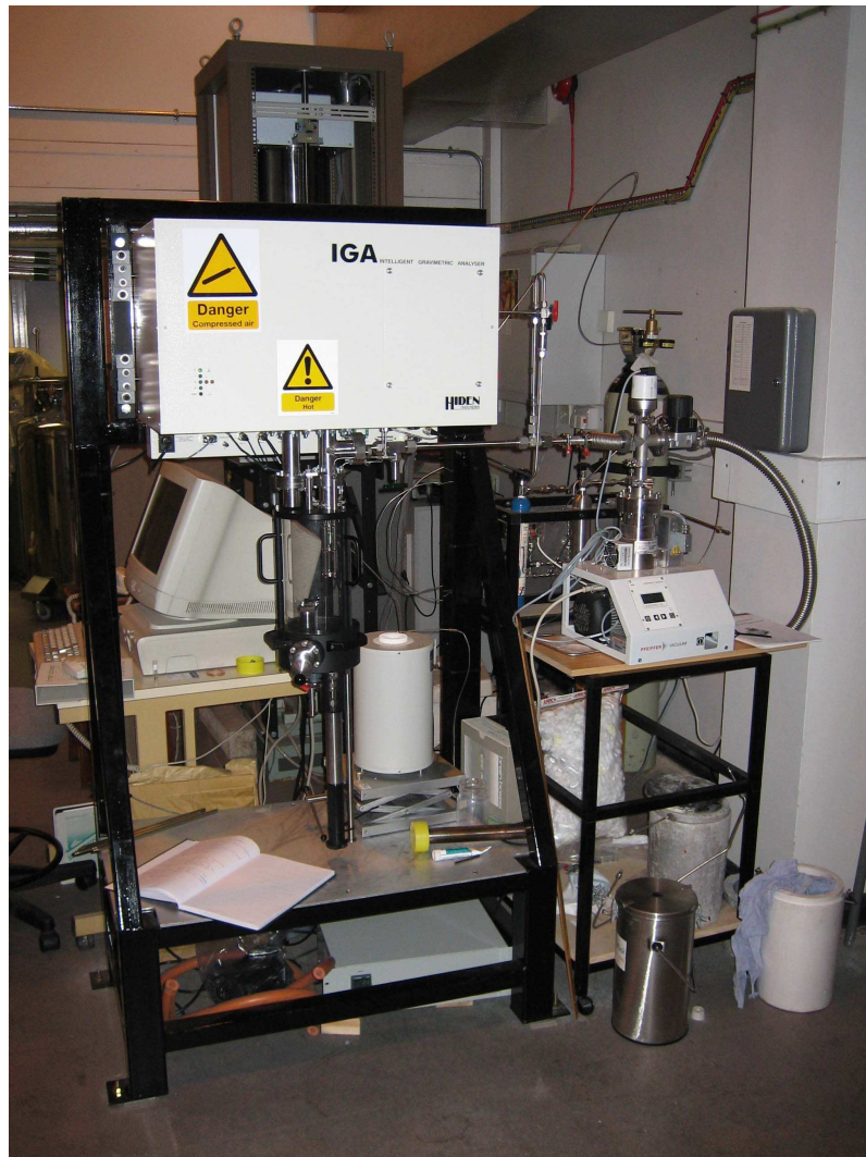
Figure 4.7: Intelligent Gravimetric Analyser (IGA) setup with dry loader attached.
