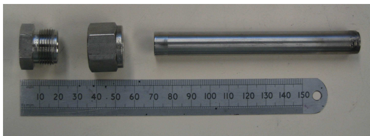
Figure 5.7: 1/2" stainless steel Swagelok tube with blanking unit for Li-alloy synthesis
