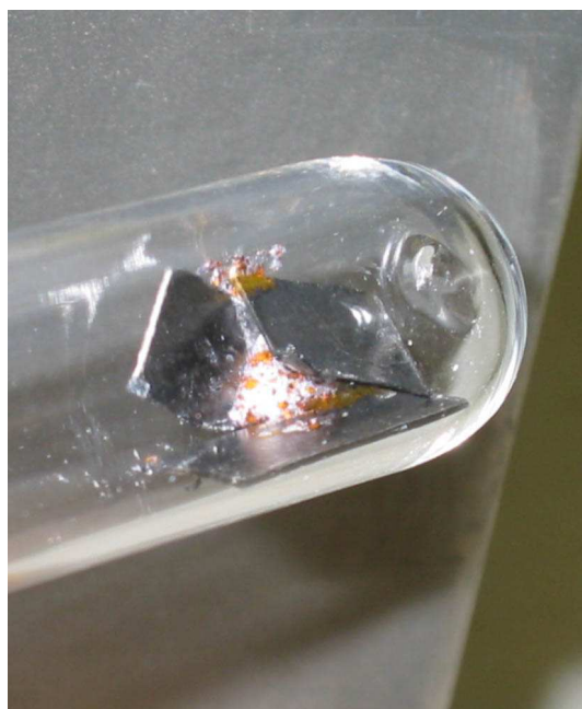
Figure 5.5: Melted potassium begins to intercalate immediately into graphite; a golden orange colour shows areas of stage-1 intercalation
