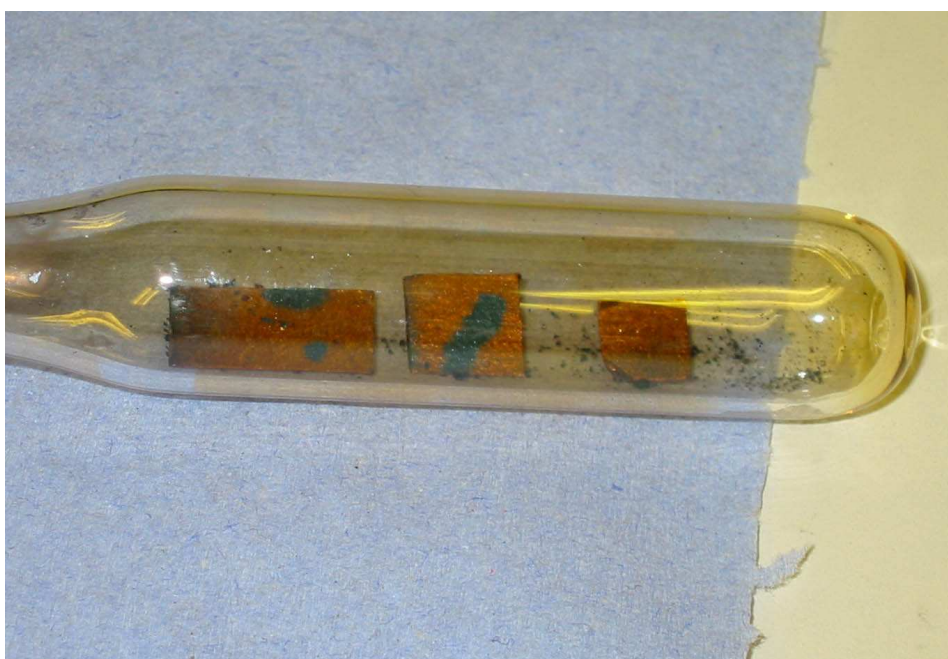
Figure 5.6: Stage-1 K-GIC with admixture of stage-2 domains
