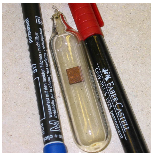
Figure 5.3: Quartz ampoule with KC 8 sample
