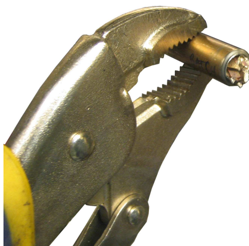
Figure 5.8: Finished \text{CaC}_6 samples embedded in the Li alloy in a freshly-opened reaction tube
