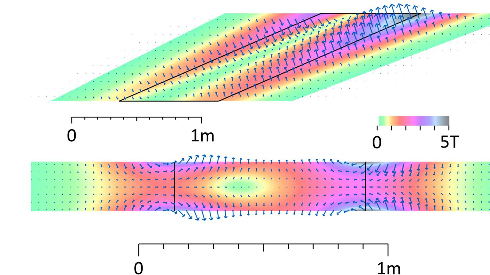
Above: Cross-section of the 5GeV ring magnet's field in ZY (top) and ZX (bottom) planes. The beam travels left to right and the orbit moves upwards on the top picture with increasing energy.
