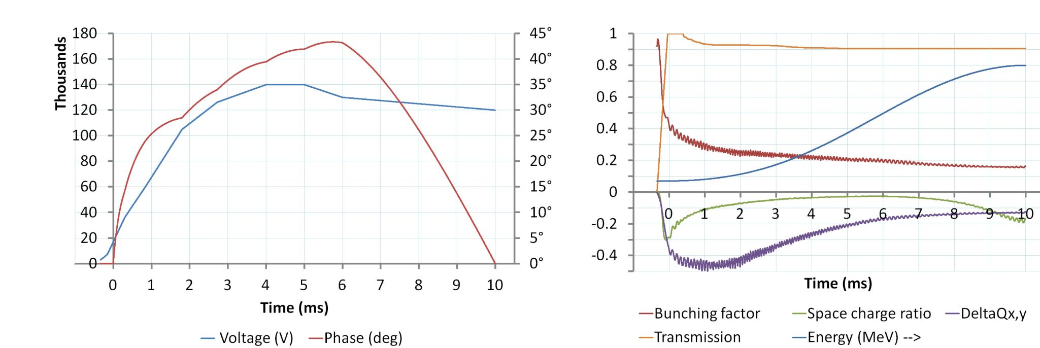
Above: To obtain an input distribution for the VFFAG (and as a check), 1D simulations were first run on ISIS starting from the linac injection at 70.44MeV. (left) ISIS first harmonic RF program. (right) Bunching factor, transmission and intensity-dependent effects in the ISIS first harmonic simulation.
