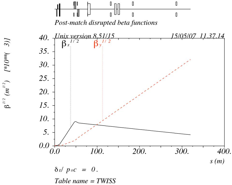
Figure 1: The  $\beta$ -functions for the 500 GeV extraction line.
