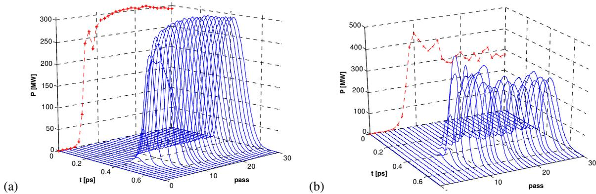
Figure 6. FELO simulation of the VUV-FEL at 10eV and cavity length detuning of 18μm with (a) zero electron bunch arrival time jitter and (b) jitter of ±80 fs. The red points show the peak intensity of the pulse at each pass.
