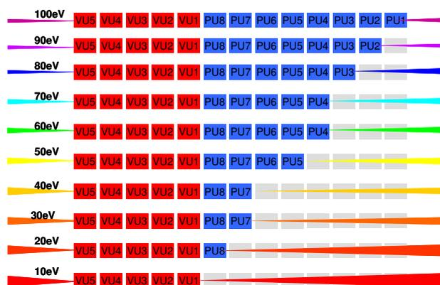
Figure 3. Schematic of the modular undulator system of the XUV-FEL demonstrating the different modes of operation across the photon energy range 10-100 eV. Electron beam transport is right to left. The minimum required undulator gap decreases in gradual steps from 28 mm for PU1 down to 10 mm for PU8 and the variable polarisation modules VU1-VU5.
