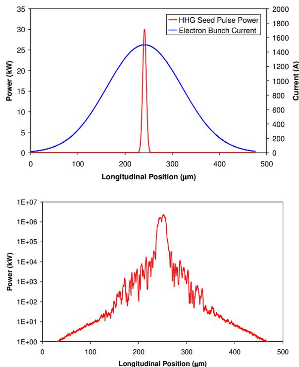
Figure 4. (a) Input HHG seed power (FWHM 30 fs) and electron bunch current as a function of longitudinal position (linear scale) and (b) radiation power (FWHM ~50 fs) at the exit of the XUV-FEL (log scale).
