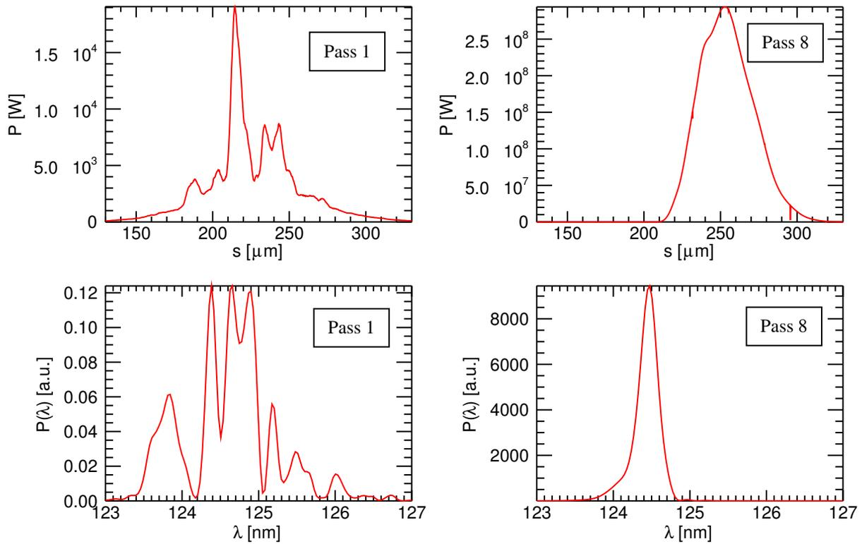
Figure 5. Genesis 1.3 [19] simulation of the radiation pulse power and the radiation spectrum after one and eight passes through the VUV-FEL for a cavity detune of 12μm.
