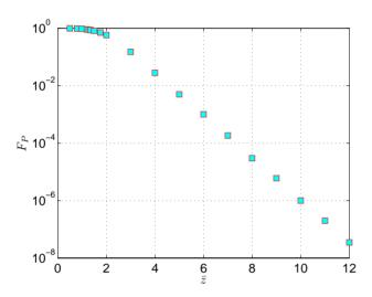
Figure 2: Results of one-dimensional steady-state simulations to determine the feedback factor  $F_P$  that maximises the output power. A fit to the numerical data over the range  $3 \le \bar{z} \le 12$ , gives  $F_P \approx 25 \exp(-\sqrt{3}\bar{z})$
