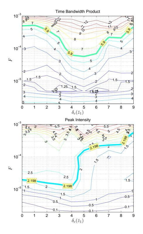
Figure 4: The complete data for all simulations, in each case averaged over 200 post-saturation pulses, for time-bandwidth product  $\langle \Delta \nu \Delta t \rangle$  (top), and peak intensity  $\langle |A|_{\text{peak}}^2 \rangle$  (bottom). In each plot the vertical axis gives the feedback *F* and the horizontal axis the cavity detuning  $\delta_c$ . The bold contour represents the averaged value seen for the 200 SASE simulations.
