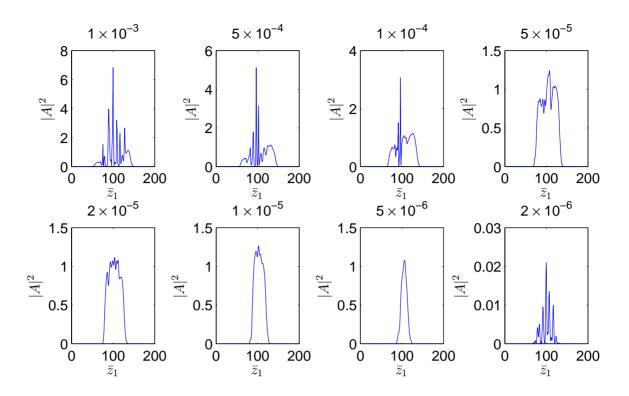
Figure 3: Typical output pulses of the low feedback RAFEL system. The feedback fraction is shown above each plot, and varies from  $F = 1 \times 10^{-3}$  (top left) to  $F = 2 \times 10^{-6}$  (bottom right). The cavity detuning value is  $\delta_c = 6.0$  for all pulses.
