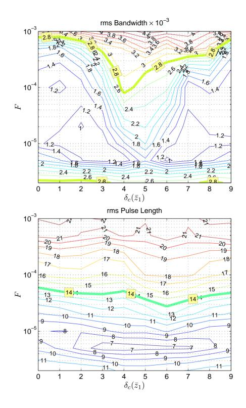
Figure 5: The complete data for all simulations, in each case averaged over 200 post-saturation pulses, for rms bandwidth  $\langle \sigma_{\lambda}/\lambda \rangle$  (top) and rms pulse length  $\langle \sigma_{\bar{z}_1} \rangle$  (bottom). In each plot the vertical axis gives the feedback F and the horizontal axis the cavity detuning  $\delta_c$ . The bold contour represents the averaged value seen for the 200 SASE simulations.
