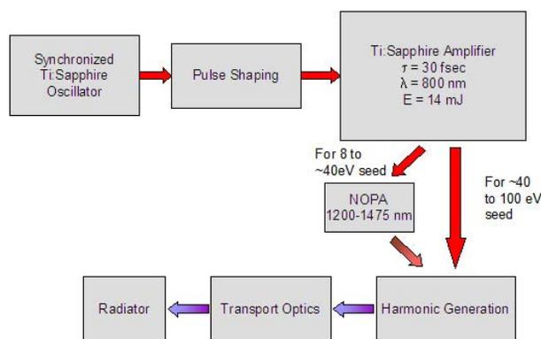
Figure 2: Diagram of HH seeding for the XUV-FEL.
