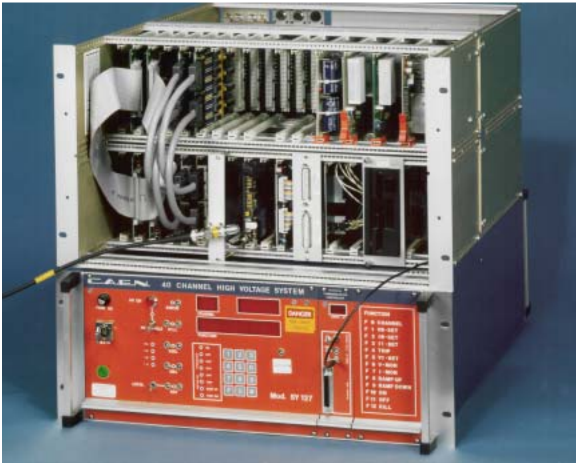
Figure 3.2: The MAC-G64 and CAEN crates. The MAC-G64 crate (on top) consists of a G64 bus below a MAC bus. The G64 bus contains, from left to right, a double-card CAEN interface, two digital input/output cards, a G64-ethernet interface connected to thinwire ethernet, a CPU card with two RS232-C connectors, and a disk controller and drive. The MAC bus contains a double-card CAEN interface, two digital input/output adapters, and the power supplies on the right. Below the MAC-G64 crate is a CAEN high voltage crate, connected to the G64 by CAENnet.
