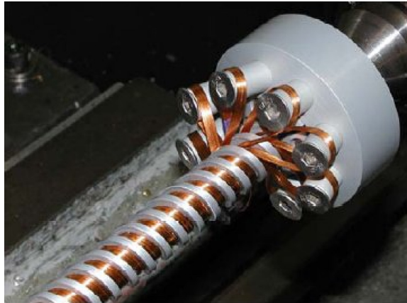
Figure 3.19: Photograph of undulator winding showing the return pegs to allow for continuous winding.
