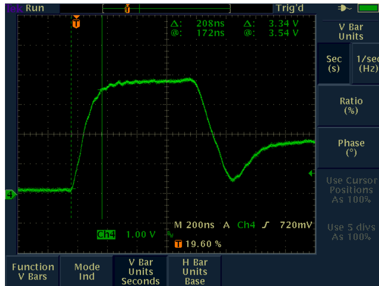
Figure 8. Measured current pulse. Time base 200 ns per cm, y axis 1 kA per cm.
