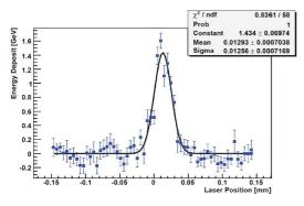
Figure 3: Convoluted horizontal size of 13 microns measured by BSM in laser wire mode in March of 2009.
