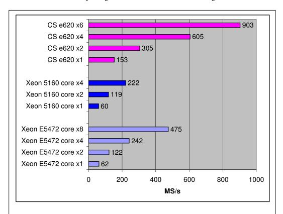
Figure 2: Performance of European option pricing on ClearSpeed e620 and Intel servers.
