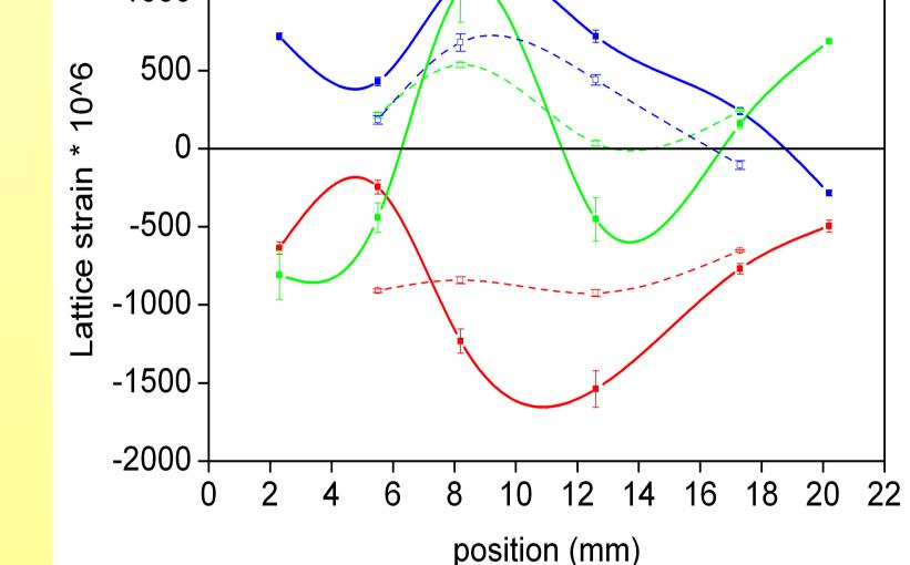
Tensile residual along the strains blade axis and compression residual state in one of the transverse direction.
