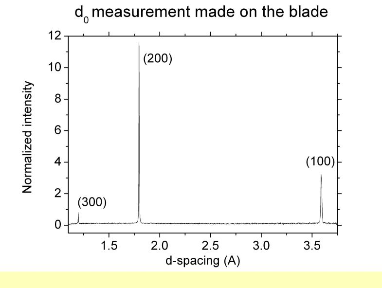
Diffraction pattern showing the (100)/(300) superlattice reflections and the (200) reflection, where diffraction peaks of both phases are overlapping.
