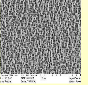
**Rafting occurs during the** thermal cycle after Solution Heat Treatment (SHT)
