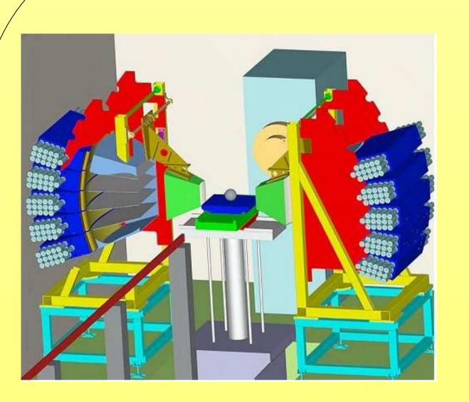
**ENGIN-X (ISIS)**: Time-Of-Flight neutron diffractometer
