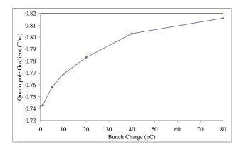
Figure 8: Gradient of quadrupole ALICE ST1-QUAD-01 (T/m) (in ALICE prior to the extraction dogleg) at 35 MeV and a range of bunch charges, after using GPT to rematch in the presence of space charge.
