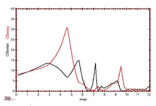
Figure 5:  $\beta_{x,y}$  for the tomography section of the ALICE to EMMA injection line from GPT at 35 MeV and 0 pC. (Note that zero metres on this and subsequent plots correspond to s = 15.7 m on the MAD results)
