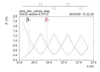
Figure 4:  $\beta_{x,y}$  for the tomography section of the ALICE to EMMA injection line.
