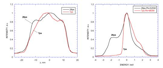
FIGURE 4. (Left) Bunch length with 7 and 28 ps laser pulses (Right)
