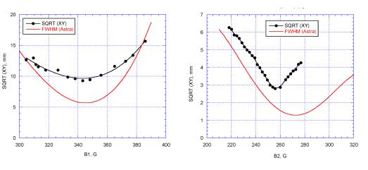
FIGURE 3. (Left) Beam size at the 1<sup>st</sup> solenoid
