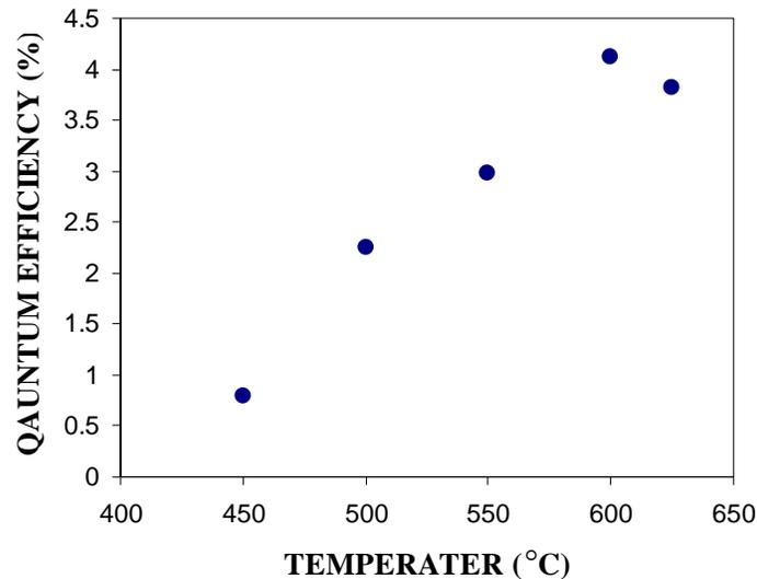
**FIGURE 3.** Quantum Efficiency as a function of heat temperature in heat cleaning procedure.
