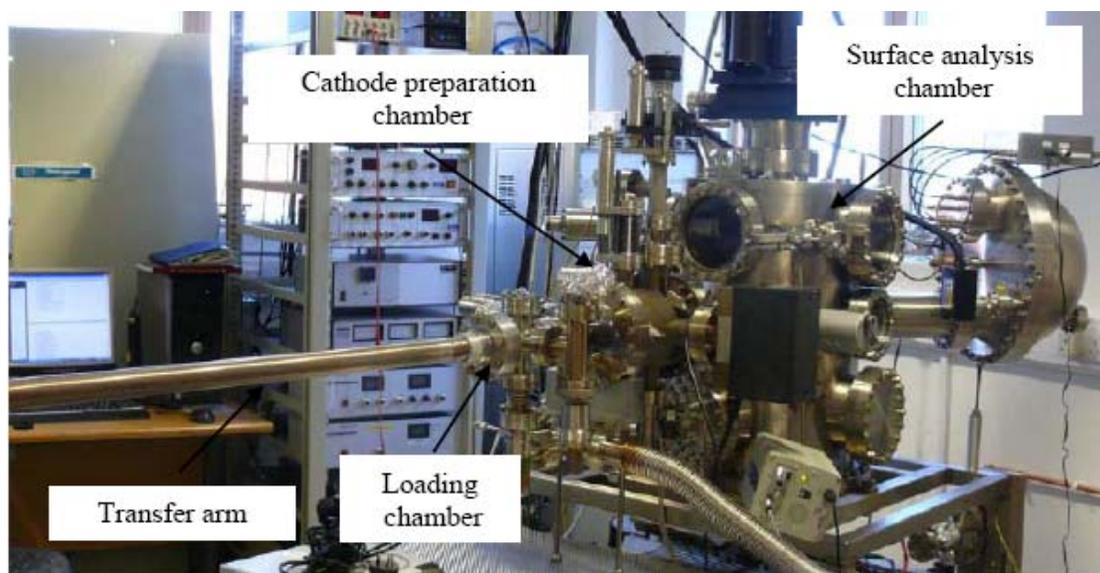
**FIGURE 1.** Picture of Photocathode experimental chamber which has been set up at the Cockcroft Institute, STFC Daresbury Laboratory.
