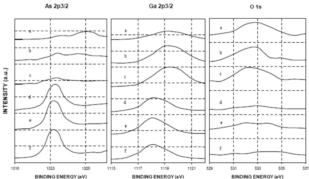
**FIGURE 2.** XPS spectra of the As 2p<sub>3/2</sub>, Ga 2p<sub>3/2</sub> and O 1s for (a) the initial dirty sample, (b) after heating to 450°C for 60 min, (c) 500°C for 60 min, (d) 550°C for 60 min, (e) 600°C for 60 min and (f) 625°C for 60 min.
