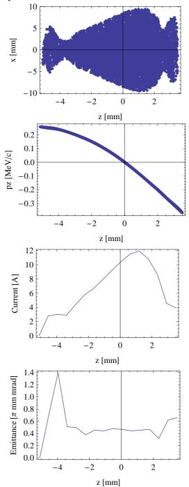
Figure 3: Beam distribution, longitudinal phase space, current profile and slice emittance for a beam after the booster cavity with zero thermal emittance.
