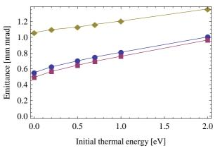
Figure 5: Emittance at the exit of the booster module against initial thermal energy. The top line is projected emittance, the middle line average slice emittance, and the bottom line emittance of the slice of peak current.
