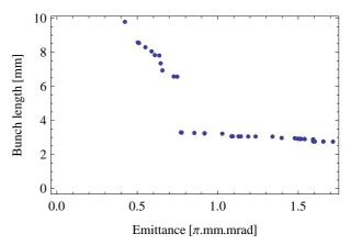
Figure 2: Projected transverse rms emittance against rms bunch length for varying the laser pulse for a 200 pC beam.
