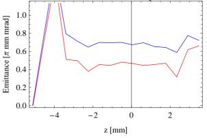
Figure 6: Slice emittance comparison between no thermal emittance (red) and that corresponding to an initial energy of 0.7 eV (blue) for Cs<sub>2</sub>Te photocathodes.
