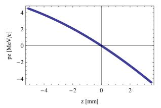
Figure 4: Longitudinal phase space of the 115 MeV bunch after the first linac module.
