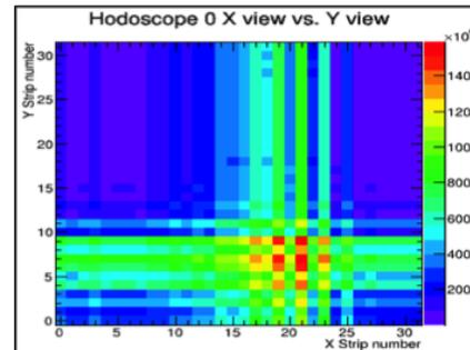
Figure 1: Muon beam intensity acquired by a scintillating optic fiber sensor.
