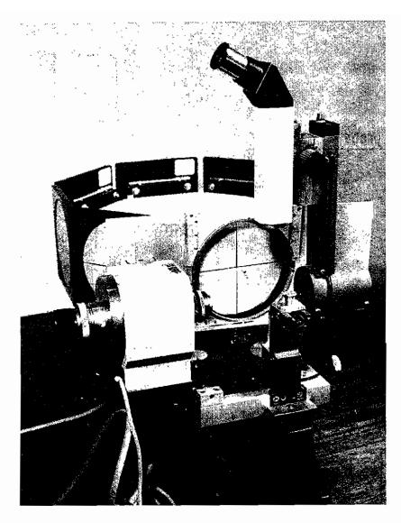
THE PHOTOGRAPH ILLUSTRATES THE 'ELEPHANT'S EARS' SCATTER GUARD ON THE ARNOT WONACOTT CAMERA. THE DEVICE WILL ONLY CUT OUT LOW ENERGY MULTIPLE SCATTERING, AND IF THE SCATTER PROBLEM IS BAD WILL PROBABLY NOT BE OF MUCH USE.
