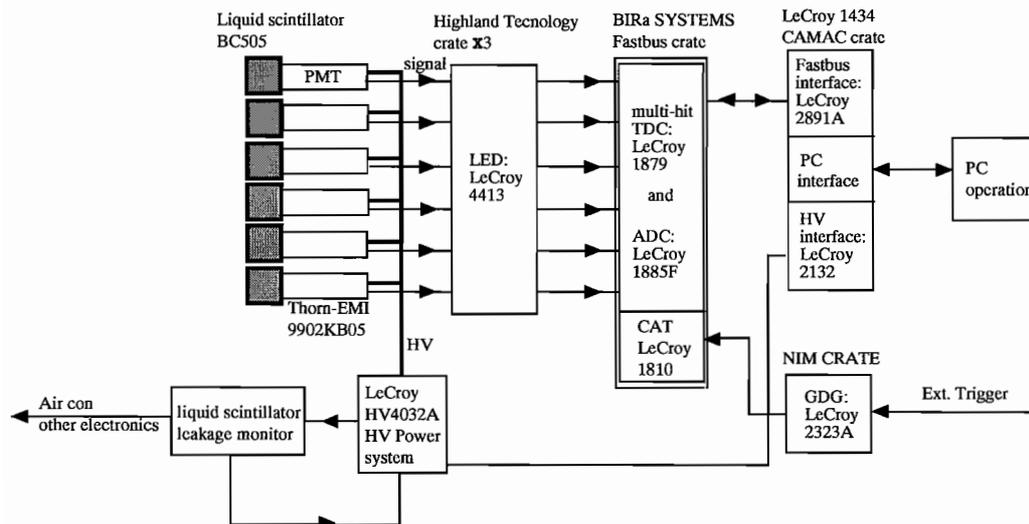
Figure A.1: Neutron detection system chart diagram.
