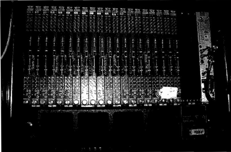
Figure 2.3: CAMAC crate with 4413 Discriminators. The power switch is next to the fan cover at the bottom of the crate.
