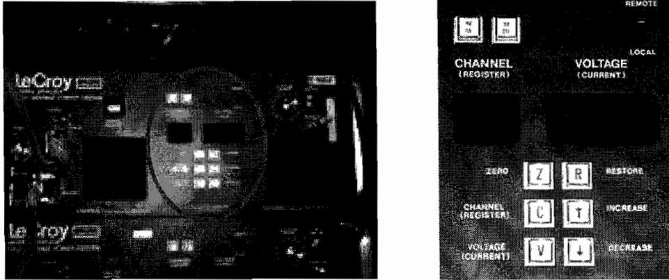
Figure 2.4: Left: high voltage supplier. Right: extended view surrounded by the red circle in the left figure. The high voltage can be set using the six keys on the bottom of the figure. Top two buttons are HV on and off button. The top right switch selects either the remote or the manual mode of HV operation.
