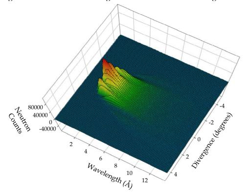
Figure 27. Vertical beam divergence as a function of wavelength for P353535
