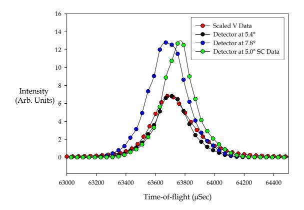
Figure 11. Effect of the non-optimal analyser profile
