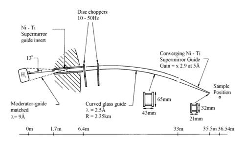
Figure 1. The IRIS Primary Spectrometer
