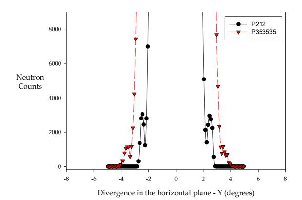
Figure 21. Horizontal beam divergence for P212 and P353535 – details at the base
