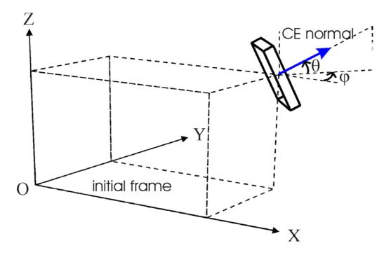
Figure 7. The definition of  $\theta$ ,  $\phi$  and Eulerian Rotation (from the Vitess user manual)
