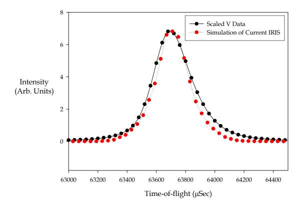
Figure 10. Comparison of the Elastic Lines - Simulated vs. Measured Vanadium Data
