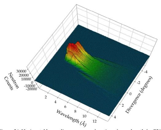
Figure 24. Horizontal beam divergence as a function of wavelength for P212
