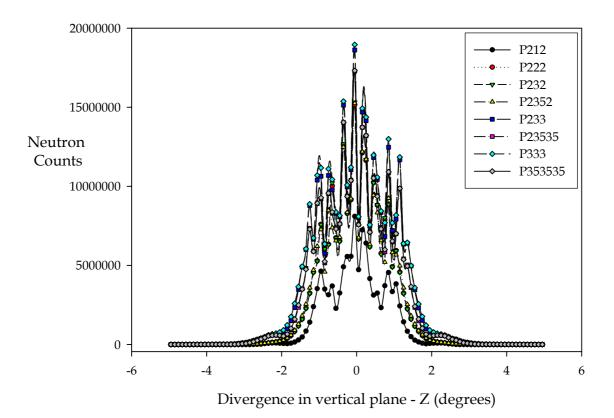
Figure 22. Vertical beam divergence for all guide configurations
