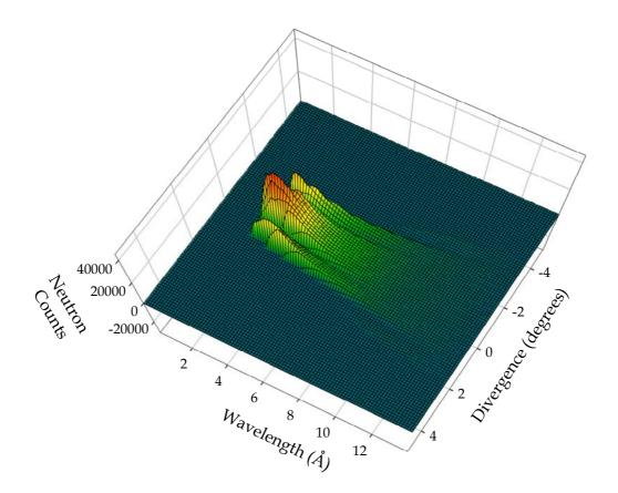
Figure 26. Vertical beam divergence as a function of wavelength for P212
