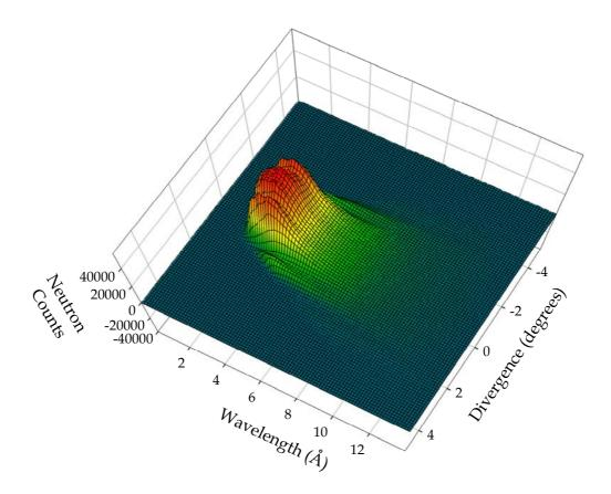
Figure 25. Horizontal beam divergence as a function of wavelength for P353535
