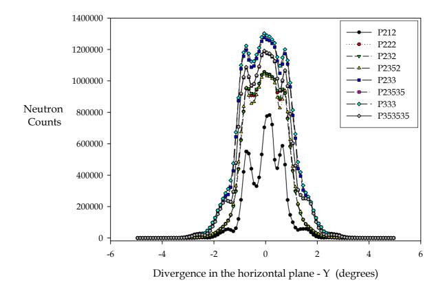
Figure 20. Horizontal beam divergence for all guide configurations
