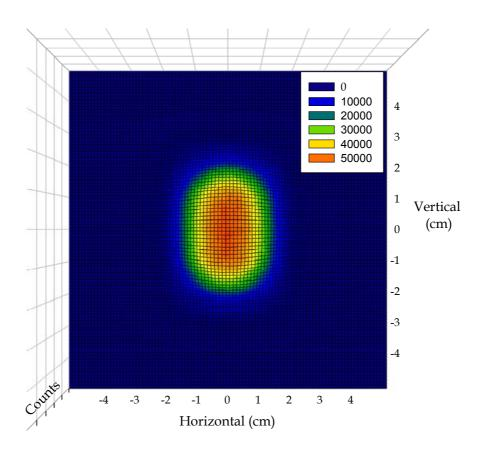
Figure 19(h). Beam profile - M333
