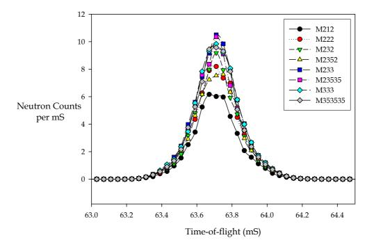
Figure 28. PG002 elastic line intensities for the different guide configurations
