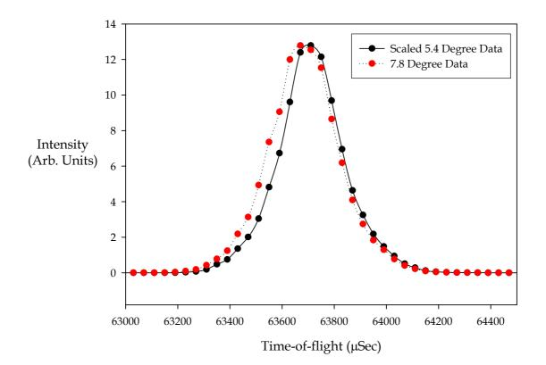
Figure 13. Comparison of Simulated Resolution Function with the Detector banks at Different Scattering Angles.
