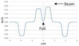
Figure 13: Longitudinal profile of the vertical magnetic field,  $B_v$  along x=y=0 axis through the injection region.
