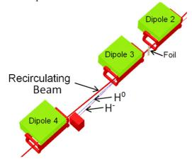
Figure 14: OPERA model of the 180 MeV injection region.
