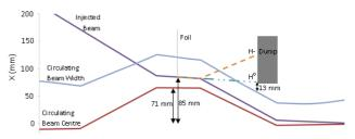
Figure 12: Geometric design trajectories for a 180 MeV injection system.
