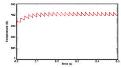
Figure 4: Temperature of the ISIS foil at 70 MeV.
