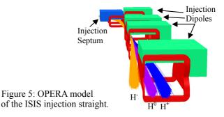
distribution at the foil position was processed with the foil interaction code described above. The resulting distributions of foil products were then tracked through the second half of the injection chicane, Fig. 5.
