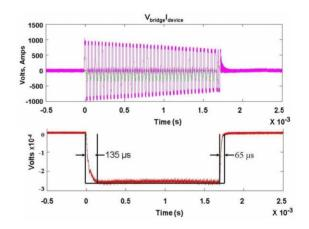
Figure 2: Top:- magenta - voltage applied by one of (three) H-bridges to one of three resonant tanks; green - current in one leg of an H-bridge. Bottom:- the output pulse profile [2], [3].
