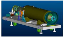
Figure 3: Schematic view of Thales TH1802 in horizontal format to facilitate placing in a tunnel [4].
