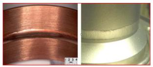
Figure 6: Examples of TIG welding on coupler components. Left: e2v Ltd [3] and right: ACCEL Instruments GmbH [9].
