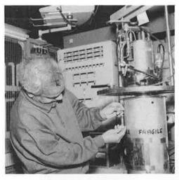
5. Load the C.C.R. into the beam using the local crane. (You must have been trained and have a RAL licence to use the crane. If not, seek HELP). Check the overall orientation with respect to the beam is correct.
