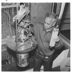
6. Replace the bolts and tighten the C.C.R. flange.
