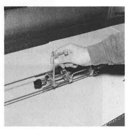
4. Connect the centre stick to the body of the furnace and connect the vacuum pipe to the centre stick.
