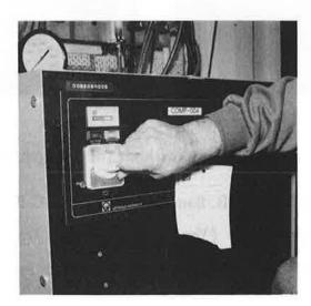
3. Disconnect the temperature control and heater connectors from the C.C.R.
