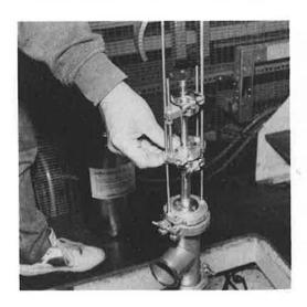
14. Connect the temperature sensors to the centre stick.
