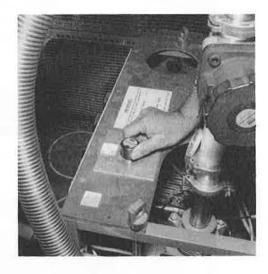
8. Open the valve connecting the pumping unit with the centre stick.
