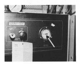
3. If the pressure is too low the compressor needs filling.
