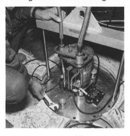
7. Pump the sample volume by restarting the Turbo Pump and opening pumping unit valve. Wait until the vacuum gauge shows better than  $10^{-3}$  bar.
