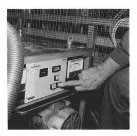
8. Connect the temperature sensors (the 4 pin plug) and heater (the 3 pin plug) to the C.C.R.
