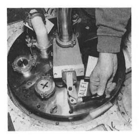
13. Lower the sample into the body of the furnace.
