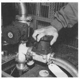
7. Switch the Turbo Pump off. Vent the Turbo by opening the vent valve on the pump for about 1 min. Close the vent valve.
