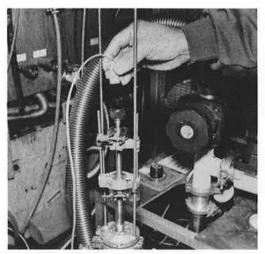
4. Lift the sample stick to the upper limit stop so that the sample is inside the detachable section of tube.
