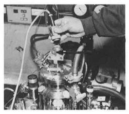
3. You must ensure at all times that air does not enter the cryostat sample volume. Therefore you have to fill the sample volume of the cryostat with helium gas. Turn the blue 'Hoke' valve pointer down. At very low cryostat temperatures (below 4K) it is first necessary to heat the cryostat to ~25K or bleed the helium in particularly slowly. (Failure to do this will cause a relief pressure valve to blow. Wasteful but not serious.) The flow meter will show no flow during this operation.
