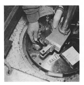
6. Close the vacuum valve which connects the pumping unit to the sample centre stick.
