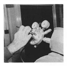
6. Purge the quick-release-coupling on the compressor with the gas from the charging line. To do this insert the coupling but do not push home, you will hear the gas escaping.
