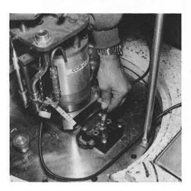
4. Switch Turbo Pump off and close the pumping unit valve. Vent Turbo by opening
