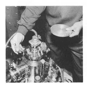
6. Quickly but smoothly remove the centre stick, and cover the sample volume with the blanking flange.
