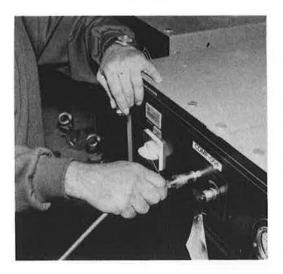
8. Set the pressure regulator to 16 bar by slowly screwing in the torque bar.
