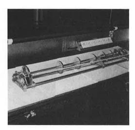
3. Attach temperature sensors (large, 4 pin plug), heaters (small, 2 pin plug) and the other auxiliary equipment necessary for your experiment. Make notes of the sensor numbers which will be entered into the computer temperature-control table.
