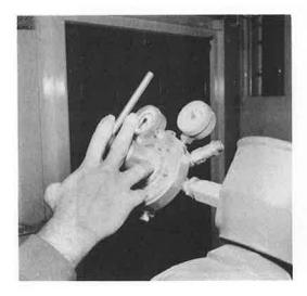
5. Open the gas cylinder valve and set the pressure regulator to 5 psi.
