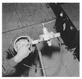
12. Disconnect charging line from the quick release coupling. For this, hold the charging pipe with one hand and with the other hand pull the quick-release-ring, away from the compressor.
