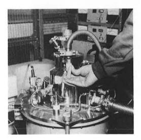
14. Pump down to the required exchange gas pressure (the vacuum gauge on the pump should show the residual pressure between 15 and 5 mbar). Return the blue 'Hoke' valve to the horizontal position. (Some users prefer to flush with helium gas via the blue 'Hoke' valve and pump down again to reduce possible contamination with nitrogen.)
