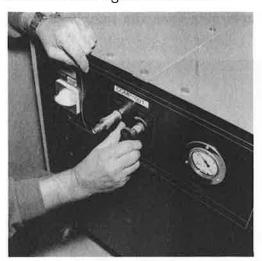
5. Disconnect the special fitting from the compressor. For this, hold the fitting with one hand and with the other hand pull the quick-release-ring, away from the compressor.
