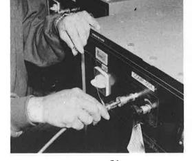
7. Fully insert the quick-release-coupling into the compressor.
