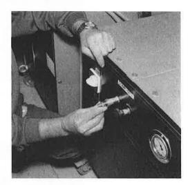
2. Reset the two buttons under the front panel of the compressor. (One button is slightly above and the other slightly below the centre of the hole.) and start the compressor.
