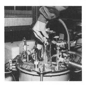
4. Wait until the flow meter again registers flow (about 5 min). The red float is spinning.
