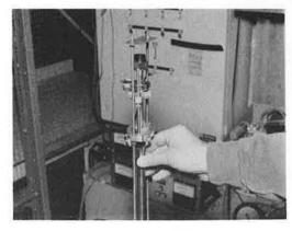
5. Close the vacuum gate valve on the top of the furnace. (If this doesn't close your sample has not been fully withdrawn.)
