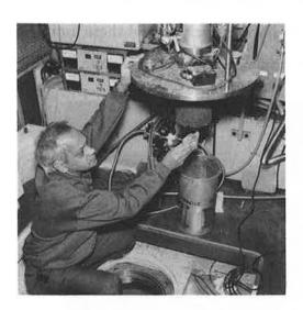
3. Attach temperature sensors and other auxiliary equipment directly onto the sample can. Make notes of the sensor numbers which will be entered into the computer temperature-control table.
