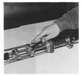
3. Adjust the position of K-type thermocouple by first slackening off the nut(s) holding it to the centre stick.
