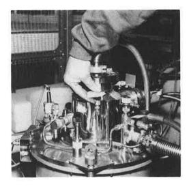
15. Connect the temperature sensor and heater connector to the centre stick.
