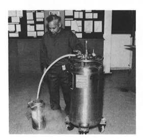
9. Immerse the sample in the liquid nitrogen and wait until the nitrogen stops boiling. (Waiting for a longer time in this operation results in a quicker overall time to achieve your working temperature.)
