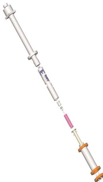
Figure 2 - Monochromatic beam Diagnostic assembly. This will give information about position, intensity and shape of the beam incident through the optics on I22.
