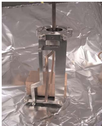
Figure 4 - Left) Primary Slits Assembly. Right) one of the water cooled blades prior to assembly.
