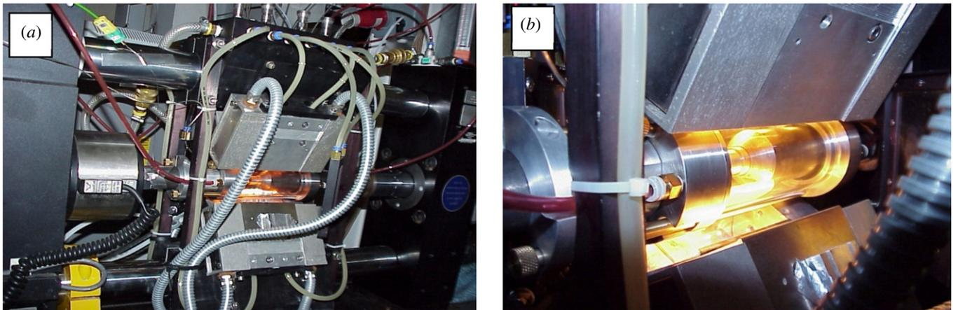
**Figure 2.** Photographs showing the previous method of providing inert atmospheres for the Engin X furnace: (a) overview of the setup and (b) close-up of the sample area and the glass canister.
