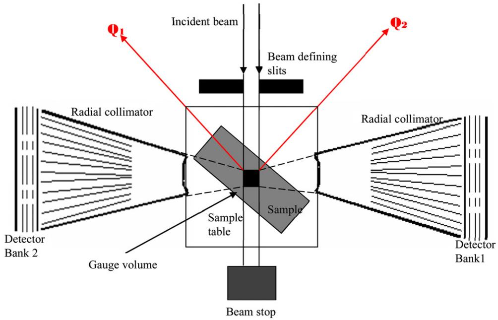
**Figure 1.** ENGIN-X experimental setup for *in situ* strain scanning. (Note that incident slits and collimators provide constraints to the maximum design size of the furnace.)
