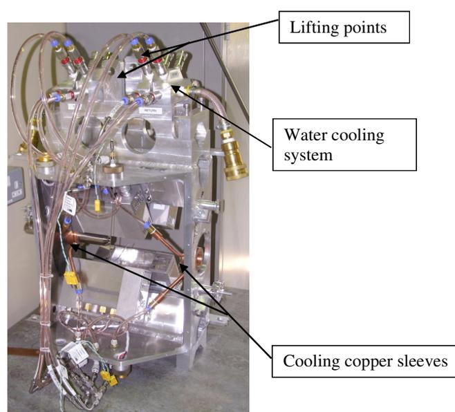
**Figure 5.** ENGIN-X inert-gas furnace off beamline, showing a compact easy-to-access assembly with lifting points cooling system providing cooling water to the lamps and cooling sleeves on the stress-rig grips.
