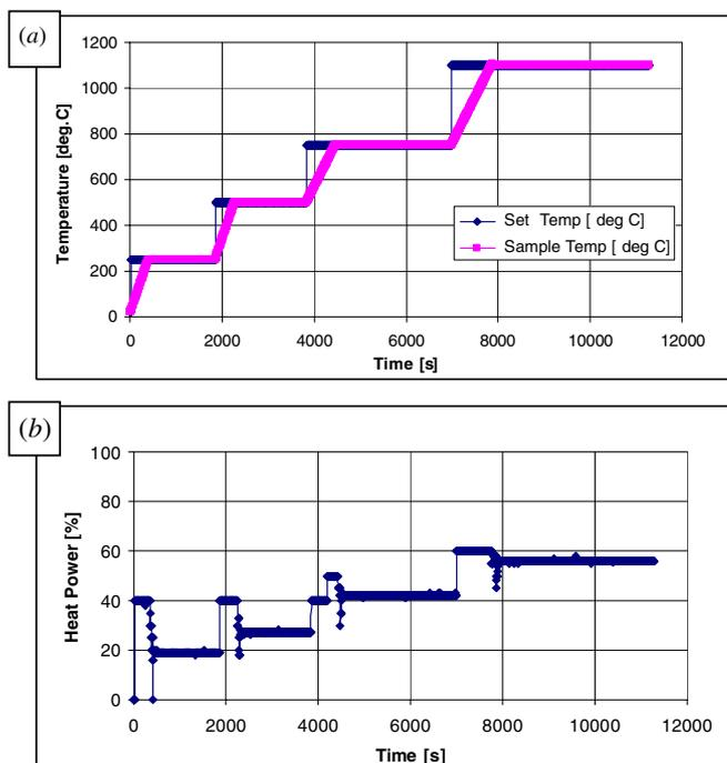
**Figure 7.** Engin-X inert-gas furnace output: (a) temperature and (b) heat output versus time on the P91 steel (9% Cr, 1% V) tensile specimen.
