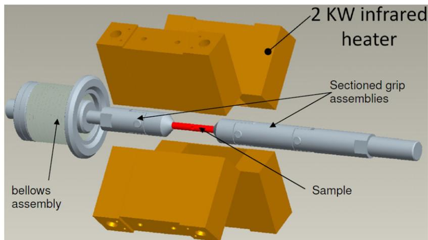
**Figure 3.** The experimental sample mounted between sectioned grip assemblies of stress rig and four 2 kW infrared heaters, positioned such that their focal zones coincide with the sample.
