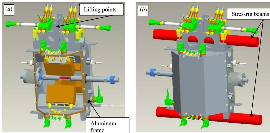
**Figure 4.** The aluminum frame that locates the heaters in position on the stress rig. (a) The assembly with all the fittings added for cooling water and power for the heaters, sensors and inert-gas feedthrough and (b) the complete assembly attached to the cross-beams of the stress rig (shown in red).
