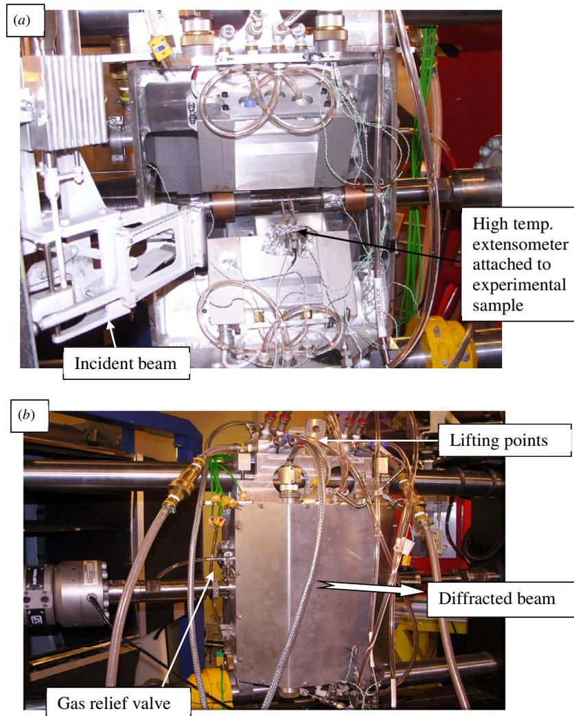
**Figure 6.** Engin-X inert-gas furnace overview of the experimental setup during the experiment: (a) incident beam side and (b) beam stop side.
