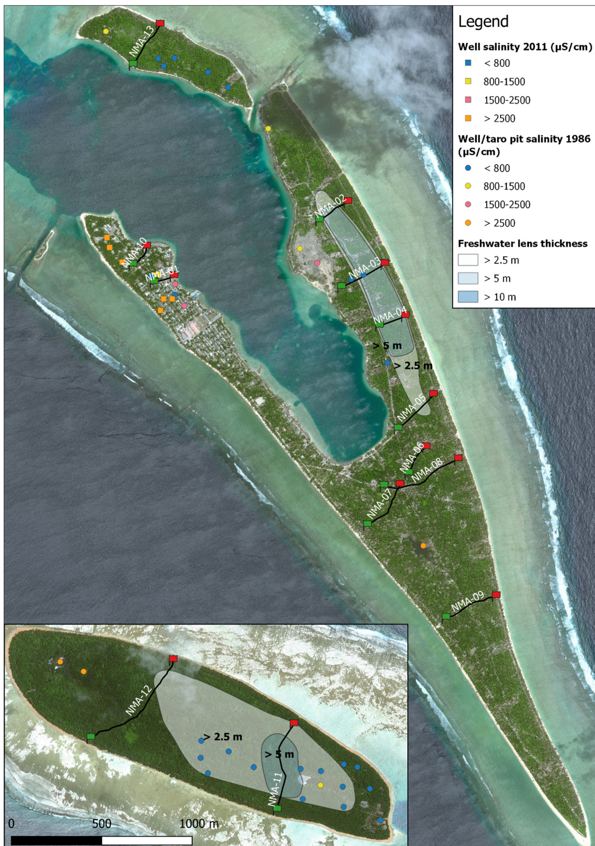
Figure 9. Isolines showing the depth to the freshwater–saltwater interface, as inferred by the electrical resistivity tomography survey lines (inset: Lakena islet).
