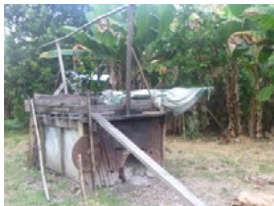
Figure 18: Peter Kope's driers are in poor condition and need to be upgraded if quality copra is to be produced (credit Moses Pelomo).
