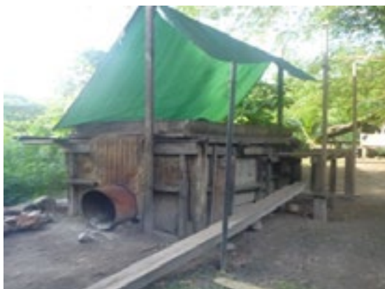
Figure 18: Peter Kope's driers are in poor condition and need to be upgraded if quality copra is to be produced (credit Moses Pelomo).
