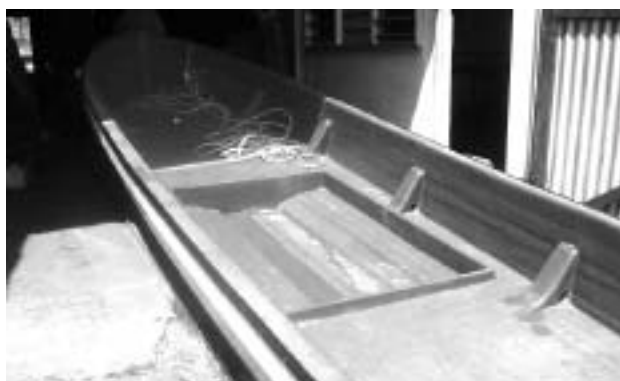
Figure 12: Inbuilt slot for the ice box in a RCFDP banana boat
