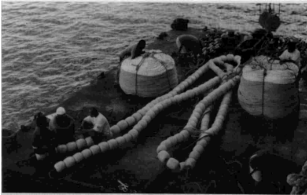
Figure 28: Loading the barge with two Indian-Ocean-style FAD systems, one on the port side and the other on the starboard
