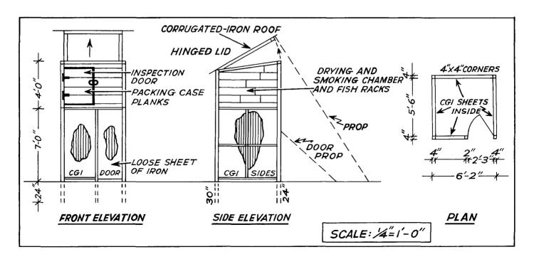
Specifications and materials: 10 sheets 7 ft. x 3 ft. corrugated iron; 3 in. x 2 in. or 2 in. x 2 in. bush poles to frame or brace iron walls and roof. Packing case timber for walls of drying and smoking chamber. One pair of large 'T' hinges and one pair of small hinges. Screws, nails, and roofing washers.
