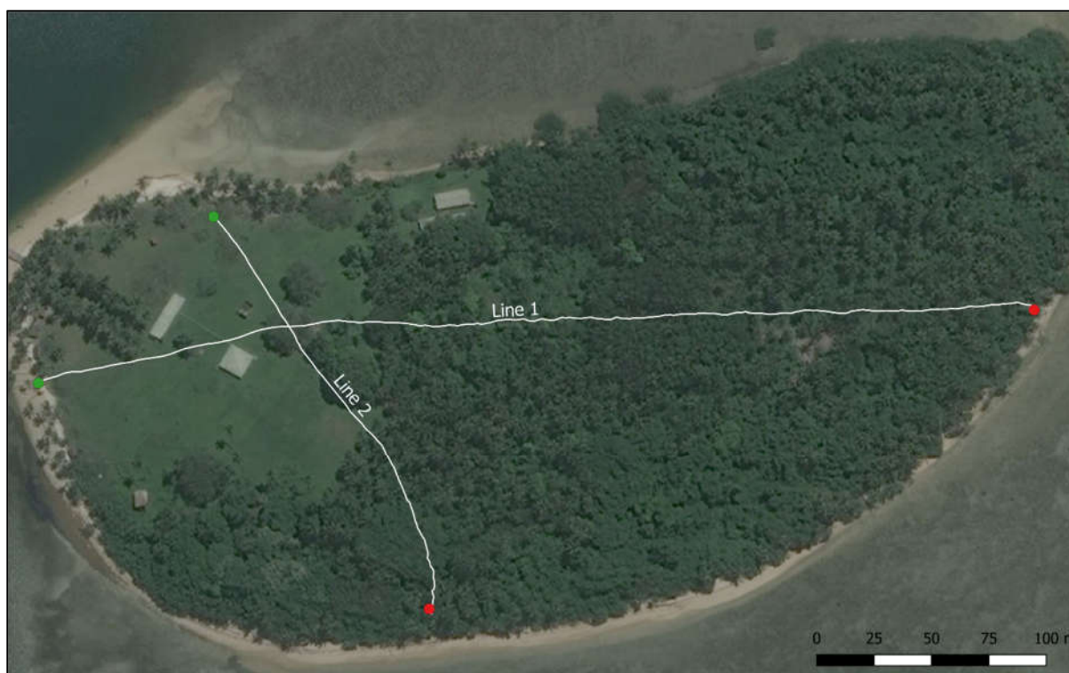
Figure 4. Test GPR profiles conducted on Nukulau island, Fiji
