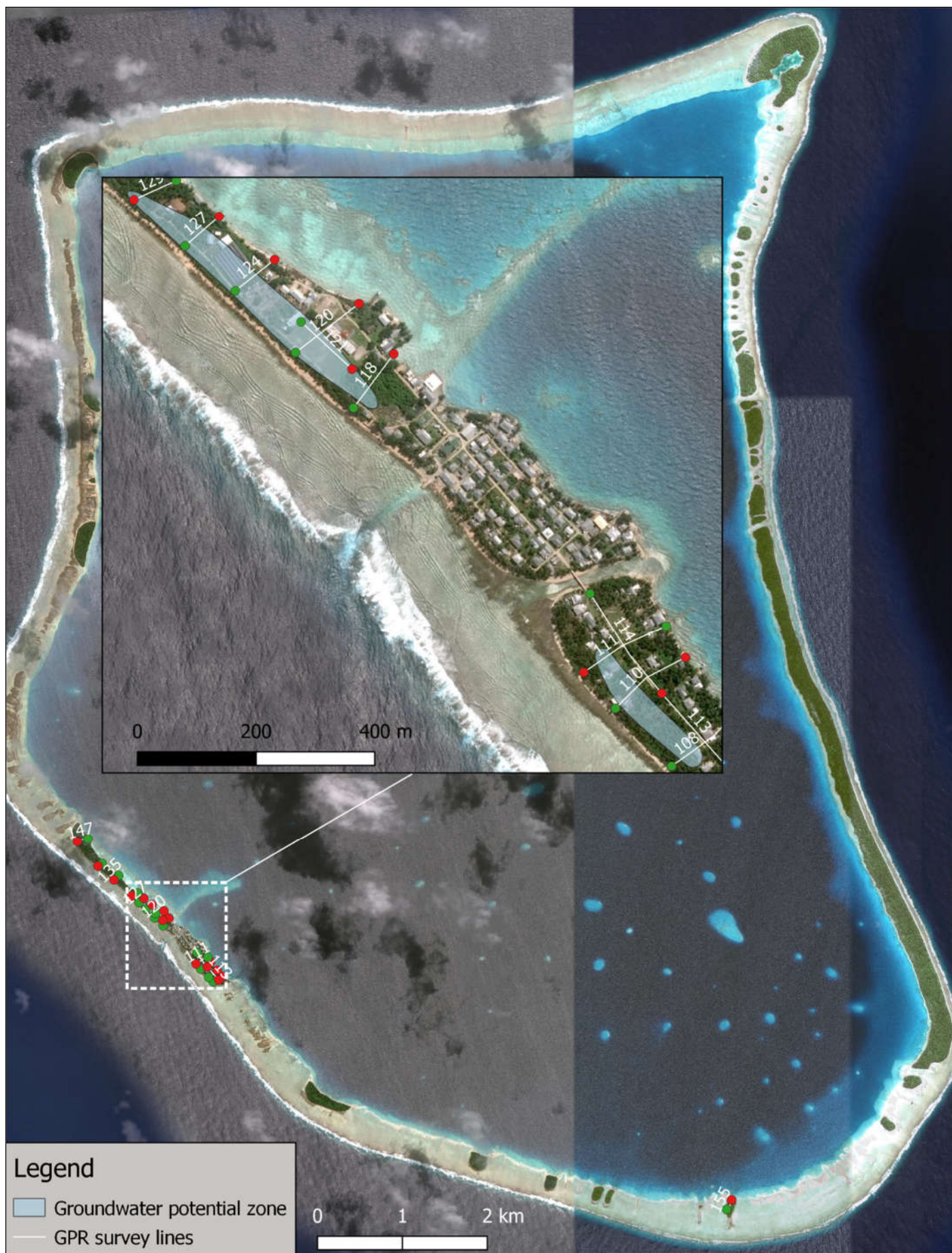
Figure 12. Nukunonu atoll - GPR survey lines and approximation of area with increased groundwater development potential
