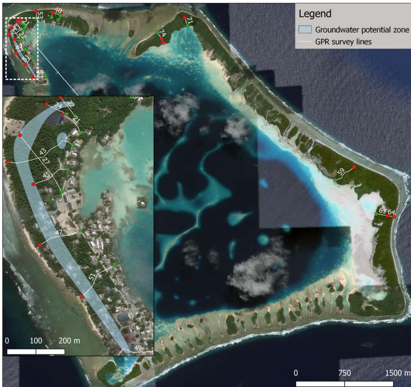
Figure 11. Atafu atoll - GPR survey lines and approximation of area with increased groundwater development potential
