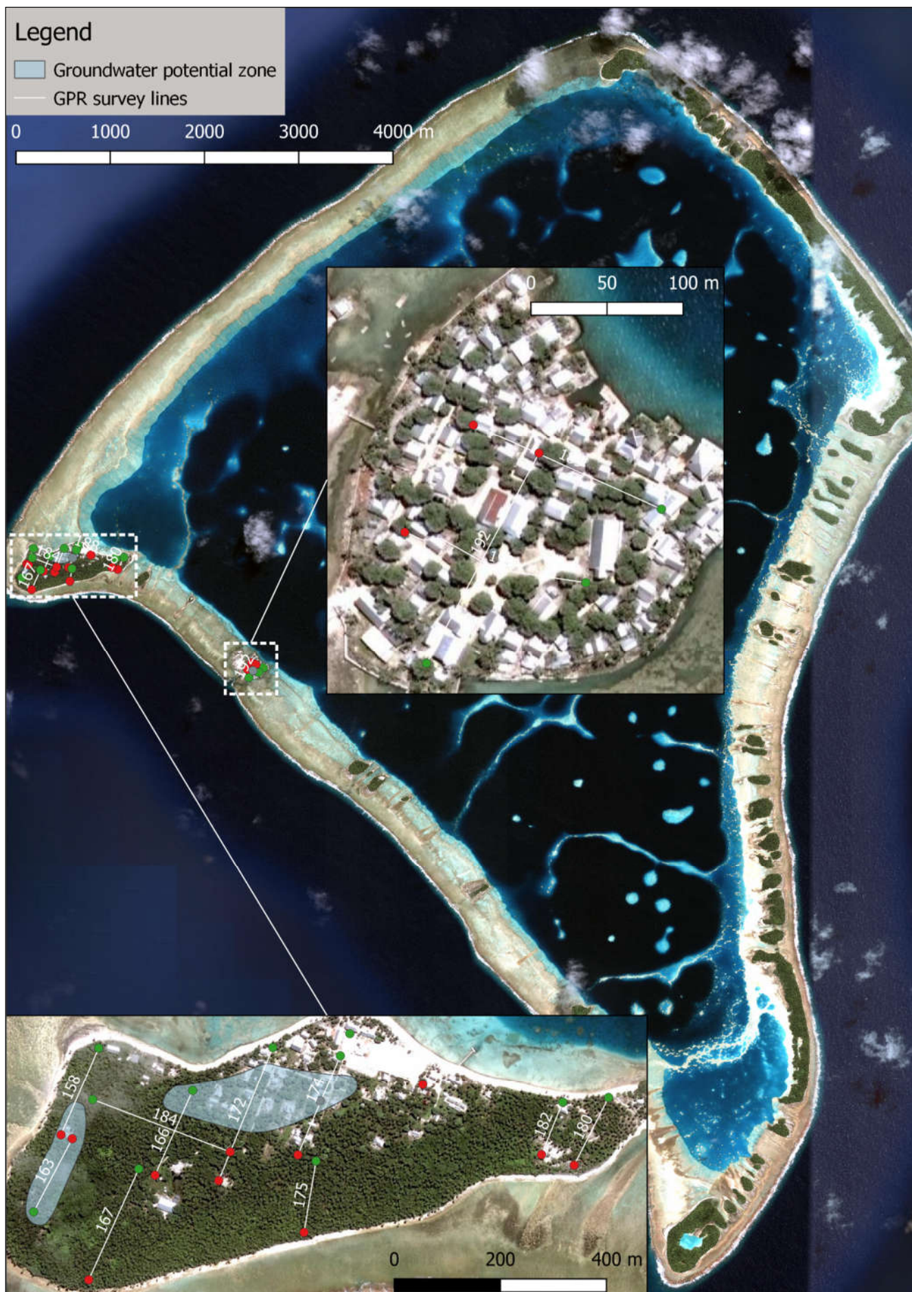
Figure 13. Fakaofo atoll - GPR survey lines and approximation of area with increased groundwater development potential
