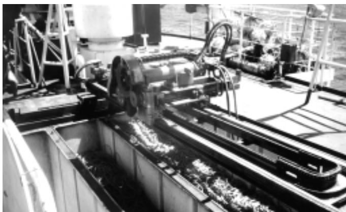
Figure 6: Transferring the mainline to the storage bin
