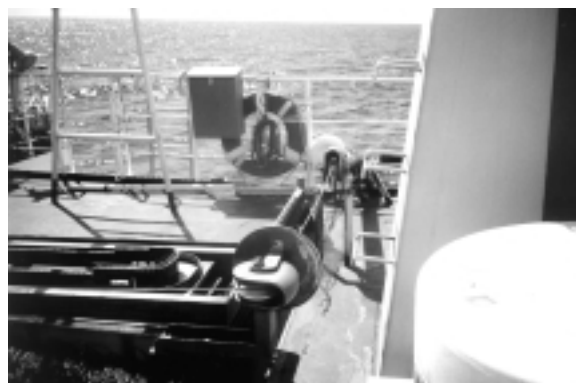
Figure 10: Hauled rope mainline being coiled onto a conveyor tray
