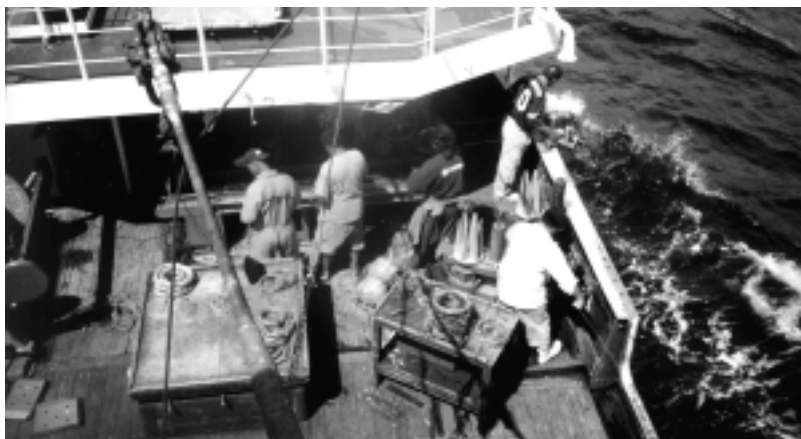
Figure 5: Hauling the rope gear, unsnapping and coiling the branchlines
