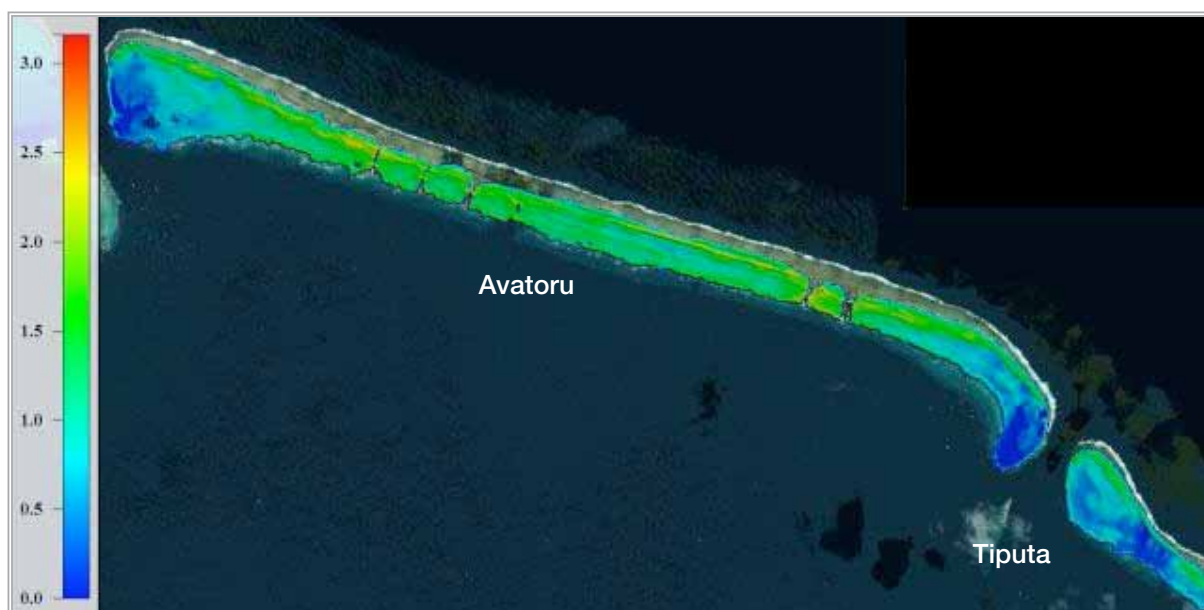
Figure 10: Speed of wave (m/second) during a storm surge event with significant wave height of 12 m. SOPAC SPC, 2013.
