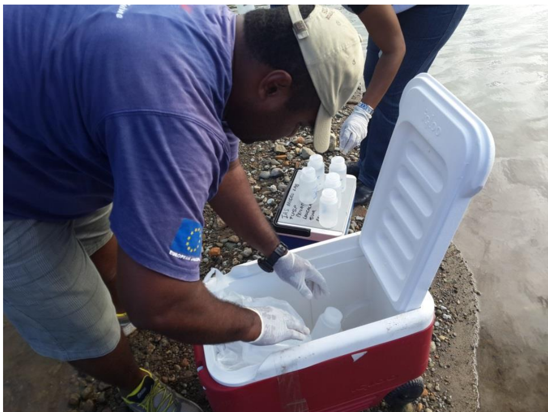
Figure A4.12. Placement of SPC sample bottles in the sanitised esky.
