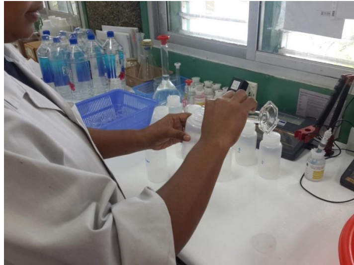
Figure A4.18. Preparing samples for 2 nd residual chlorine test.
