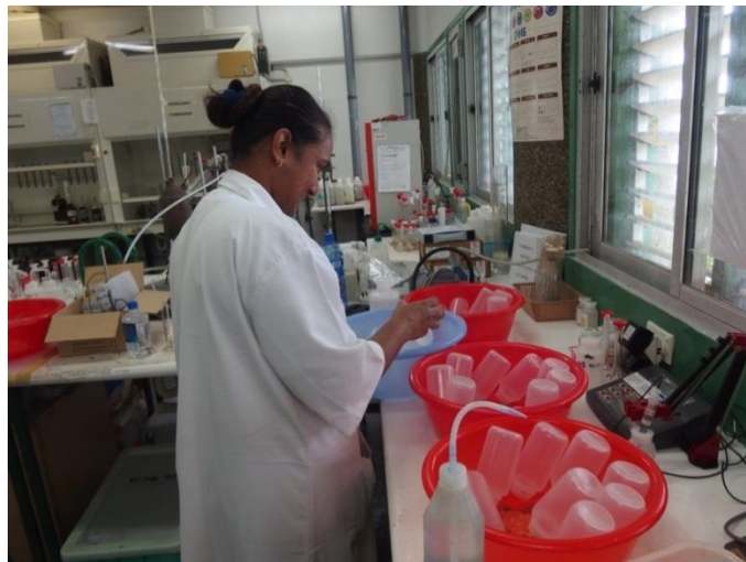
Figure A4.2. Bottles dried overnight after sterilisation process before randomly selected for residual chlorine test.
