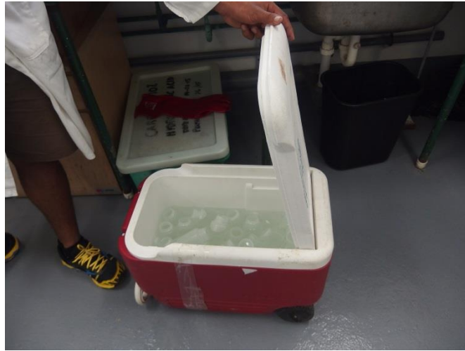
Figure A4.1. Soaking sampling bottles in a sterilised esky prior to adding of bleach solution.
