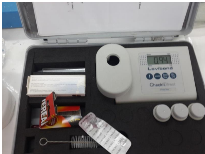
Figure A4.3. Lovibond laboratory kit and chlorine tablets used for measuring residual chlorine.
