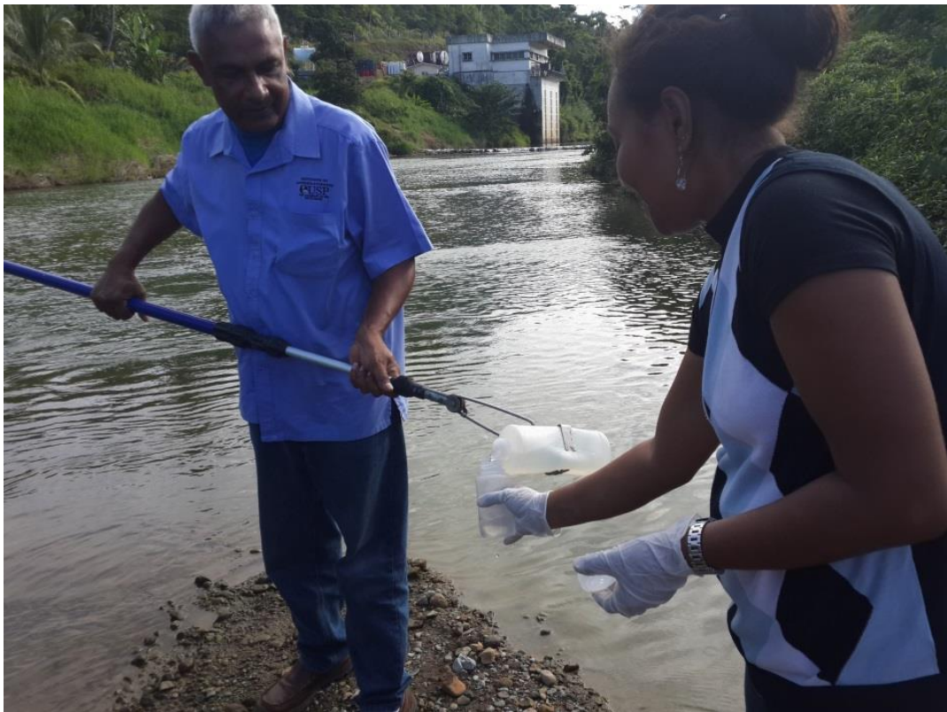
Figure A4.11. Pouring sample water into SPC bottles.
