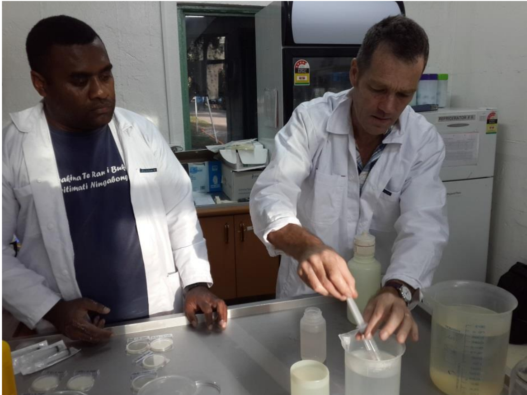
Figure A4.16. Rinsing of sterile water and running through the filter housing as a sterilisation step.
