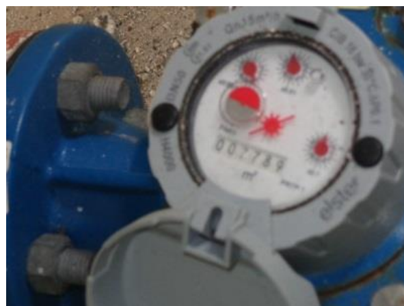
Figure 19: FFM at gallery 12 showing 7789.994 m 3 at the start of the test.
