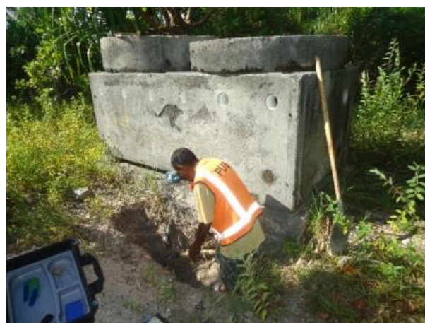
Figure 11: PUB personnel setting up UFM at gallery 12. Note that access into the pump house was prevented by the two concrete slabs.
