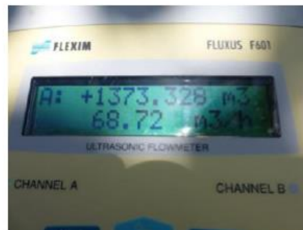
Figure 2: Water meter accuracy test at the Bonriki WTP main meter (Schwalger & Skerjanz, 2014).
