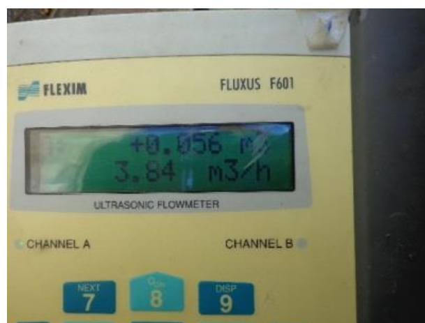
Figure 16: UFM #1 gallery 19 reading 0.056 m^3 and 3.84 m^3/h , equivalent to 1.07 L/s.
