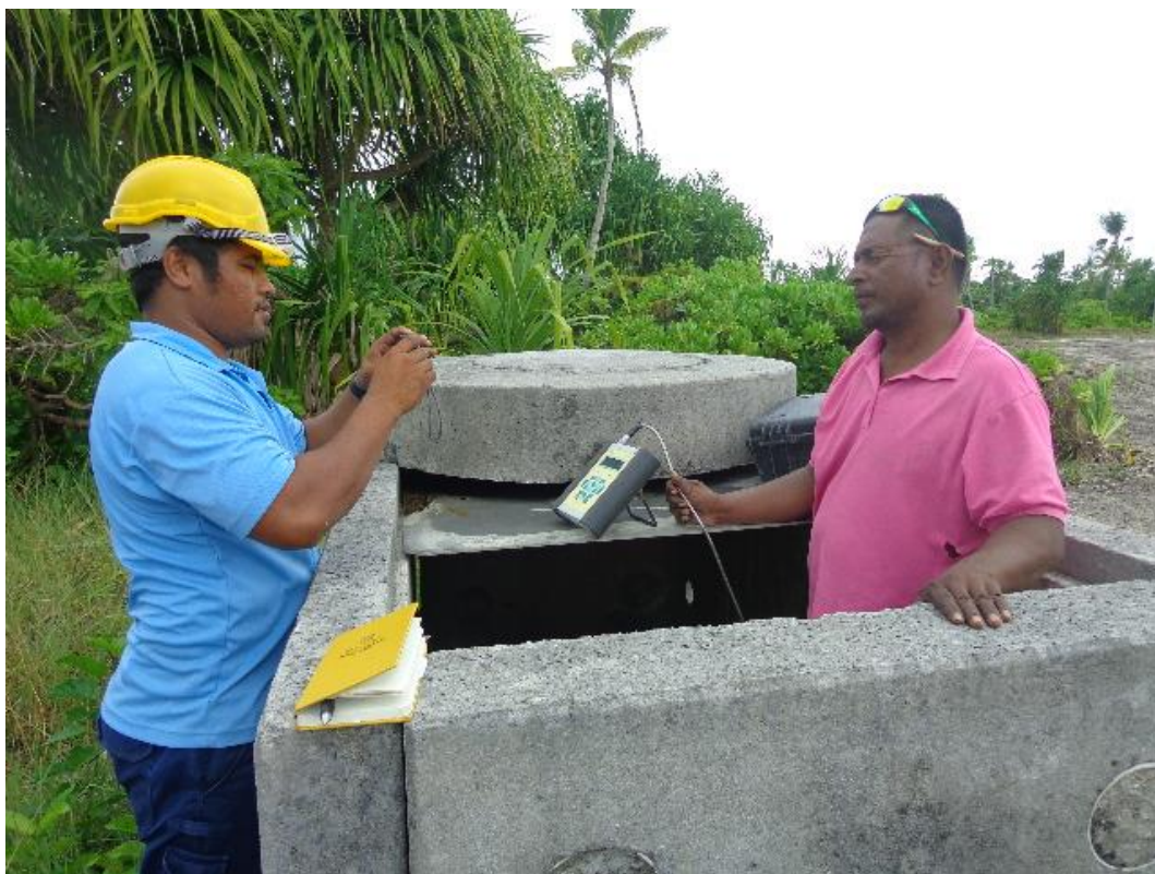
Figure A4.7: PUB staff installing UFM and taking photos at the beginning of the meter test at gallery 10.
