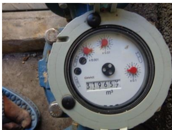
Figure 15: FFM at gallery 19 reading 319656.862 m^3 at the beginning of the test.
