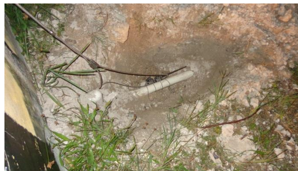
Figure 12: UFM device attached onto the PVC drainage pipe outside gallery 21.
