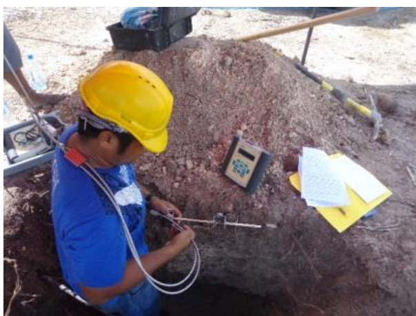
Figure 8: PUB technician setting up UFM unit 2 to test the Bonriki WTP main transmission line.
