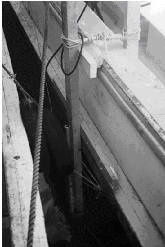
Figure 2: Transducer housing mounted on timber and lashed in place on starboard side of vessel
