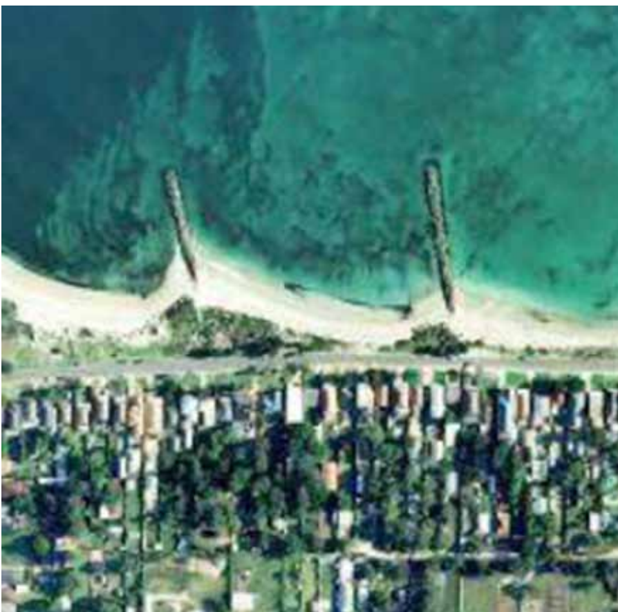
Figure 8: An aerial view of a groyne field that has successfully trapped sand to maintain the beach
