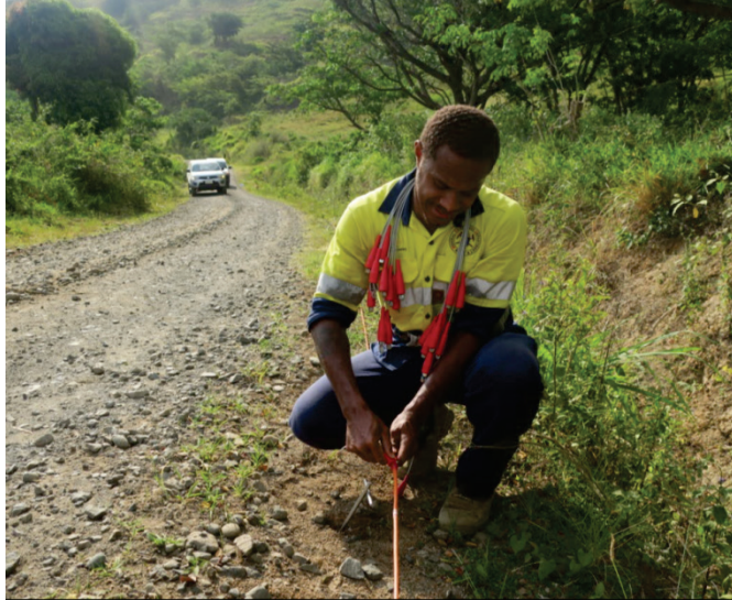
Figure A4.5.3. Attaching jumper cables to connect the electrodes and the cables.
