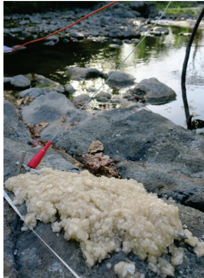
Figure A4.2.4. Using bentonite to improve electrode contact on basal volcanic exposed at a creek bed.
