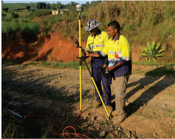
Figure A4.5.5. Elevation measurements taken along the survey transect using the Trimble R10 series.
