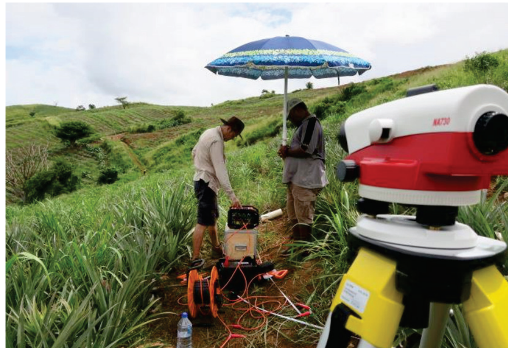
Figure A4.1.4. ABEM LS kit operated alongside the elevation survey unit.
