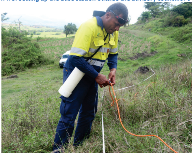
Figure A4.4. 4. Initial setup of survey line 6 where a jumper cable is used to connect the electrodes and electrical cable.
