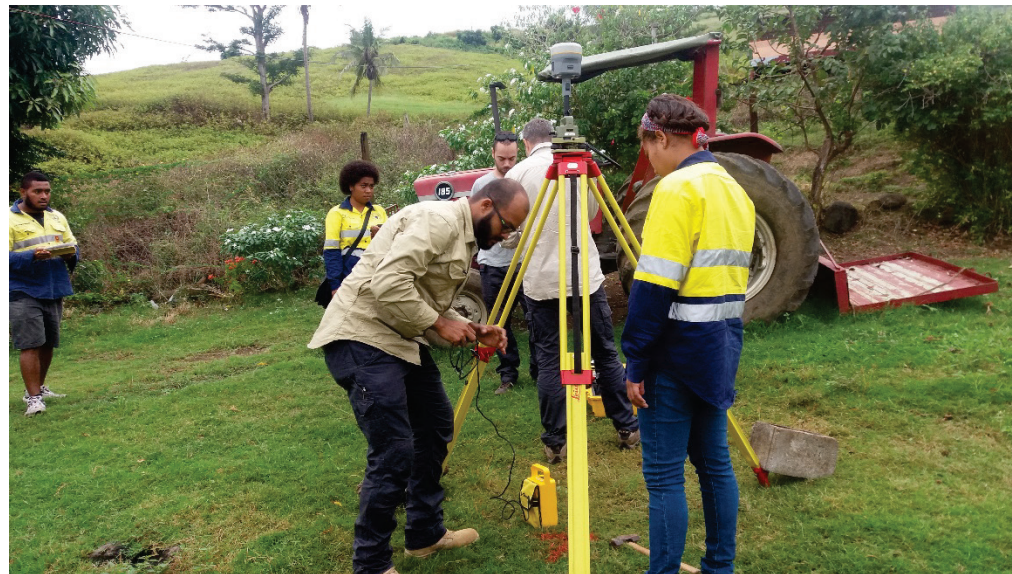
Figure A4.1.8. Setting up of the Trimble R10 base station prior to field assessment in Qerelevu in May 2017.
