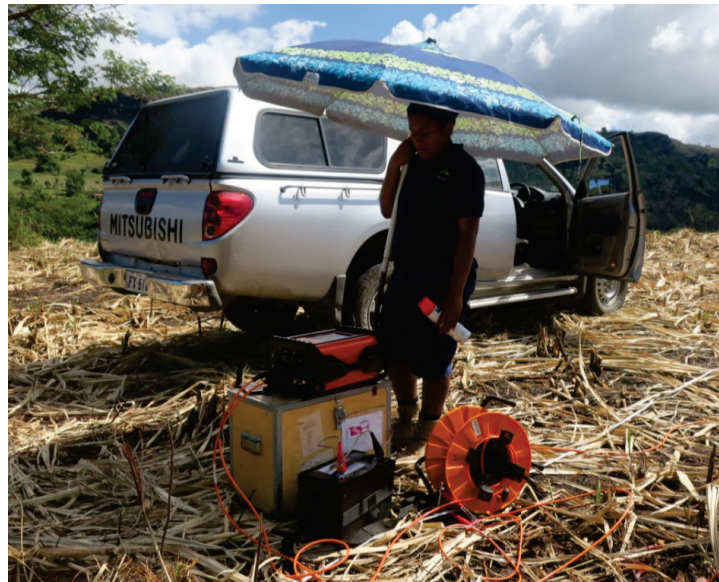
Figure A4.4. 2. ABEM LS equipment in operation along survey line 5 around Benai.
