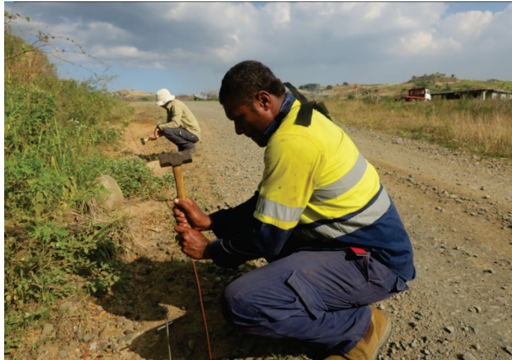
Figure A4.5.2. Hammering steel electrodes to ensure adequate ground contact.
