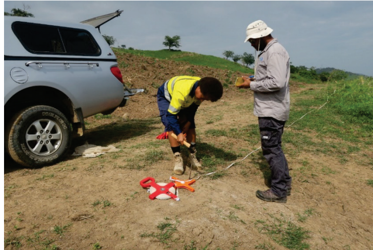
Figure A4.6.1. Setting up a survey profile using a measuring tape.
