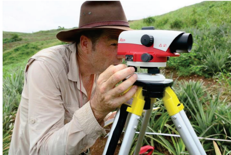
Figure A4.1.3. Dumpy level instrument used to assess relative topographical variation along the survey profile.
