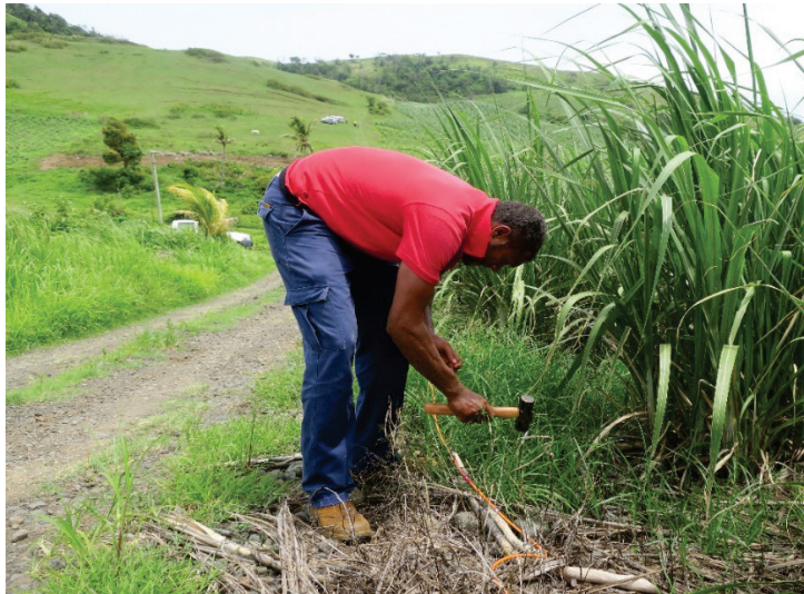
Figure A4.7.2. Hammering steel electrode into ground as part of survey profile setup.
