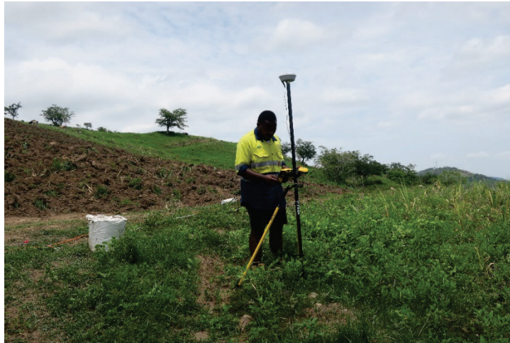
Figure A4.6.3. Trimble 600 series used to capture location and elevation measurements.
