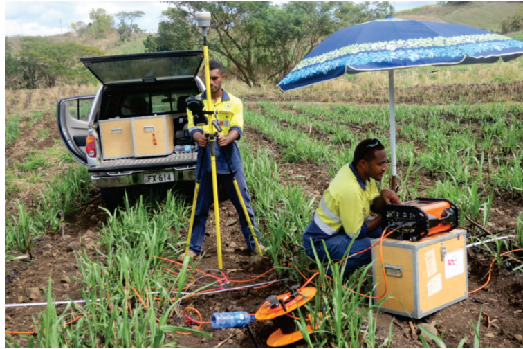
Figure A4.4. 1. Resistivity data collection conducted alongside topographical survey.
