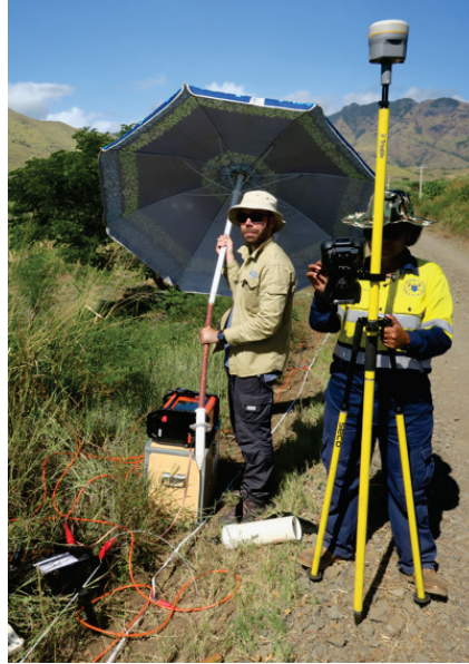
Figure A4.2.3. The team using Trimble R10 GPS during the geophysics survey.
