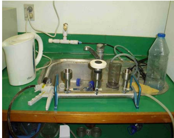
The membrane filtration used by TWB lab – that not a very clean space for bacto analysis.
