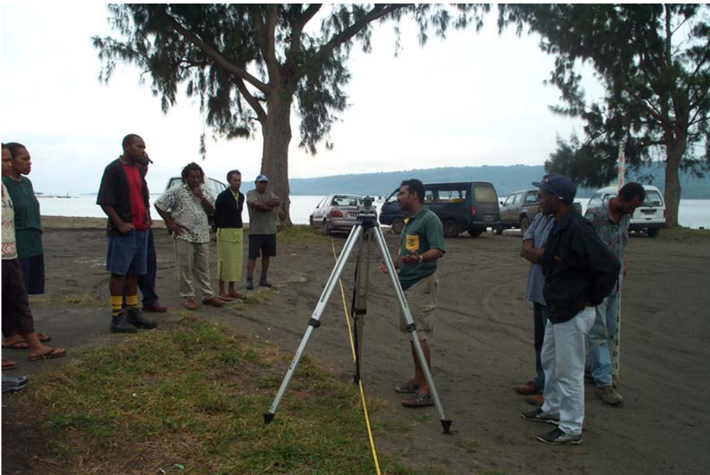
Field-survey demonstration using an automatic level and staff to carry out a beach profile survey in Mele Bay.
