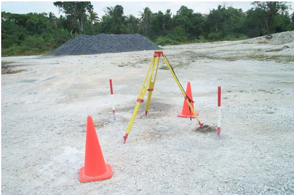
Permanent Ground Control Survey Mark (STN01) in Pango, Efaté.
