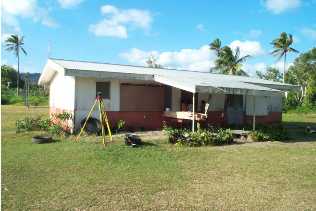
Ground Control Survey Mark, Mele_BM05, used for Beach Profile Survey occupied by GPS.
