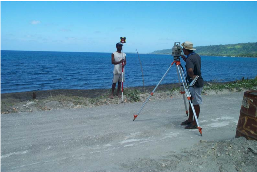
Beach Profile Survey using Sokkia Set 2C Total Station and Reflector Prism.
