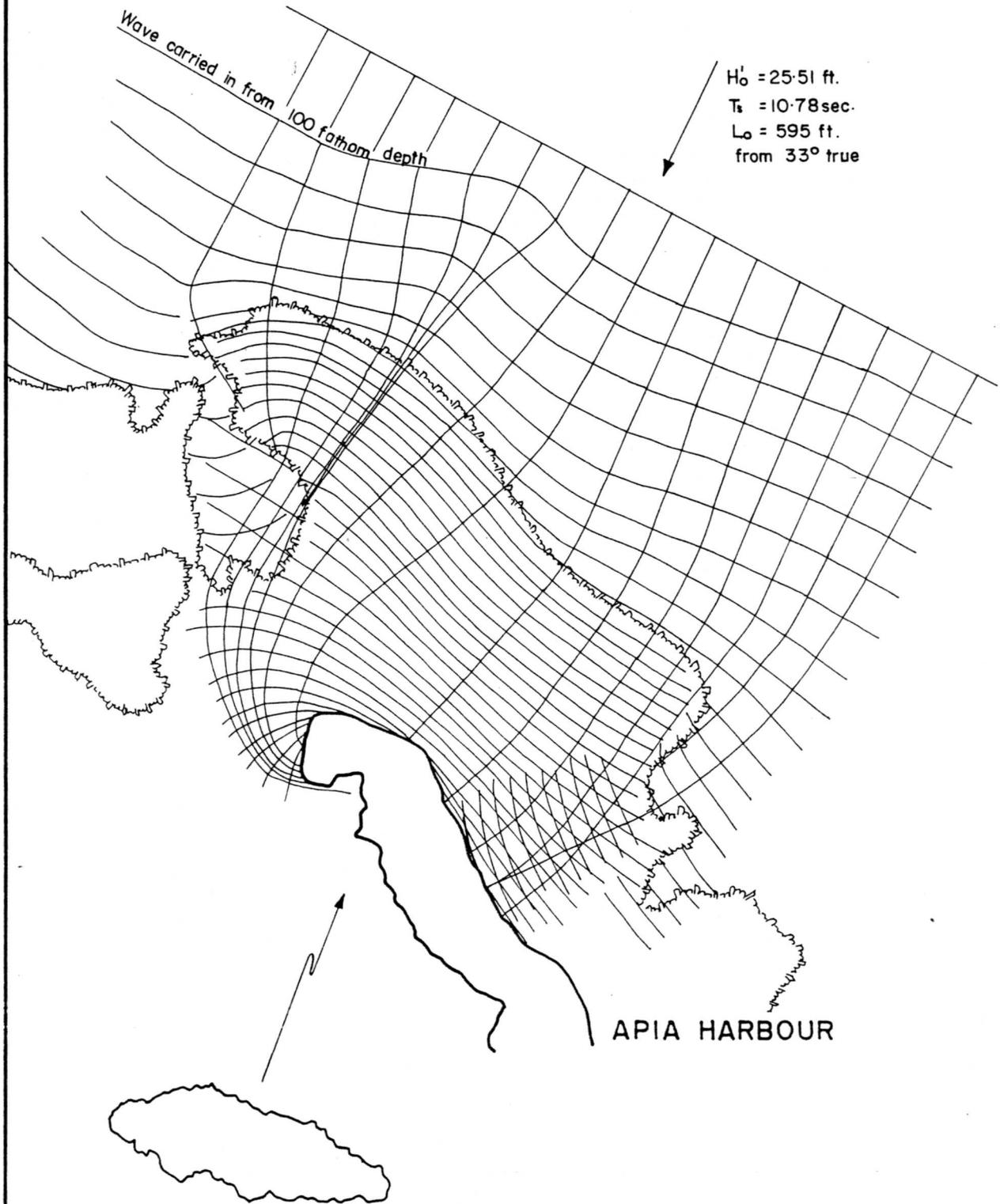
Wave diffraction of a north east wave for the Post Sand dredging condition at Mulinu u Pt. Note the high concentration of orthogonals being focussed upon the beach towards the southern end of the Point.
