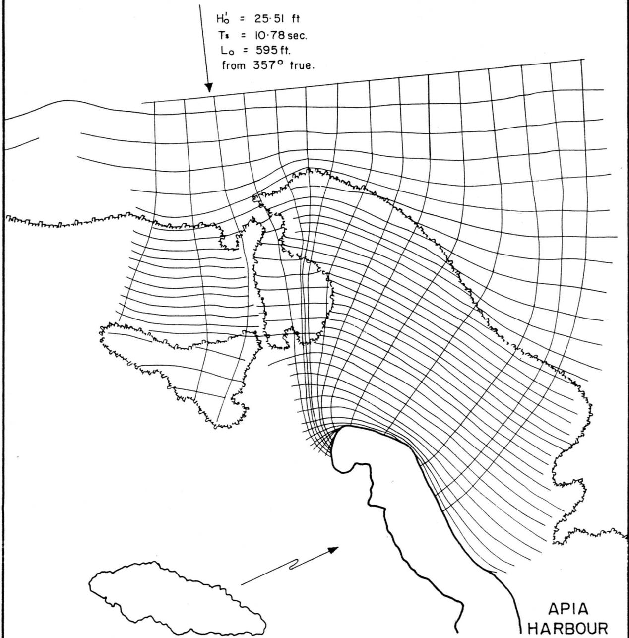
Wave diffraction of a north wave for the Post Sand dredging condition at Mulinu'u Pt. Note the in-force focusing of wave energy upon the beach at the east side of the Point.
