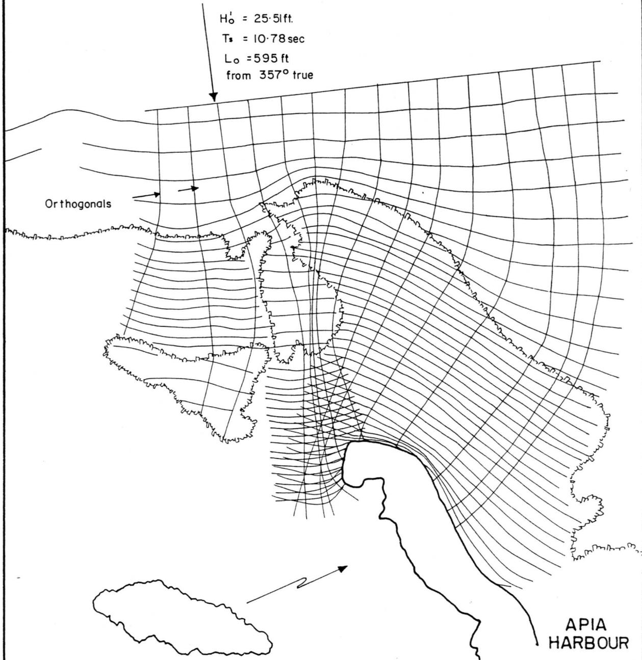
Wave defraction of a north wave for the pre-dredging condition on Mulinu'u Pt. Note moderate concentration of wave energy upon the point with a significant number of orthogonals passing to the west of the land area into Vaiusu Bay
