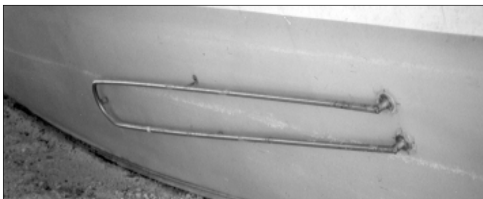
Figure 10: Keel cooling pipes on F/V Tekokona II
