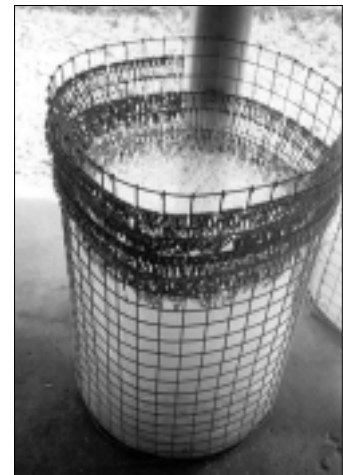
Figure 7: Branchline bin constructed from wire mesh, with branchlines
