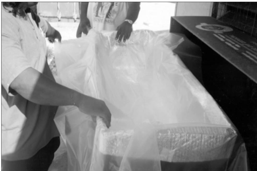
Figure 17: Assembled carton with insulation and plastic liners
