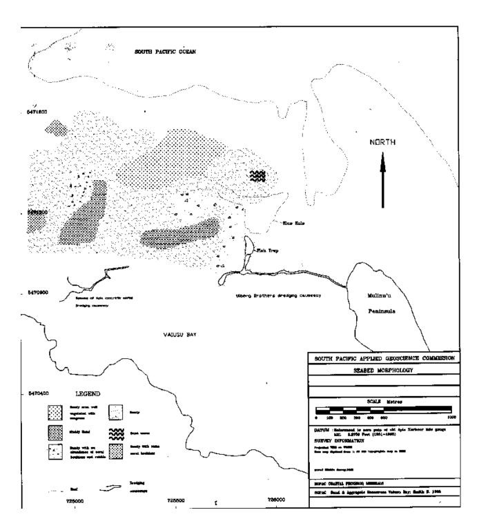
Figure 8. Seabed morphology interpreted from the jetprobe locations.
