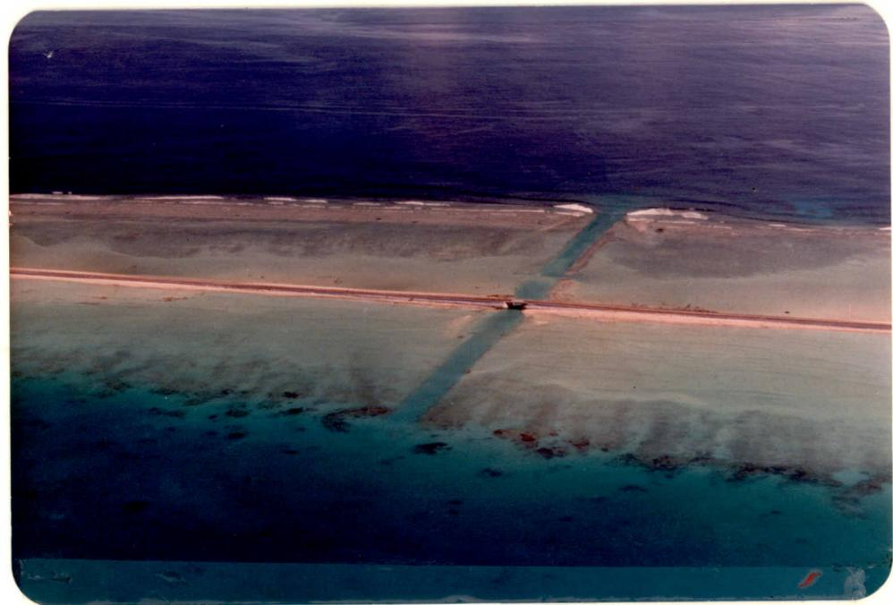
FIGURE 8 (a) Fisheries access channel looking toward the lagoon. Note the shoal area in the channel due to draining of the reef flat. Note also the greater beach width to the right of the bridge, indicating a right-to-left longshore transport (westward) on the ocean side.
