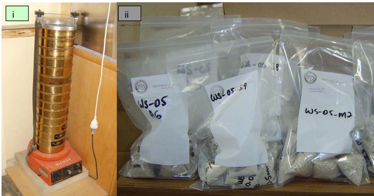
**Figure A.** The sieving process – i) the sieves being stacked on a sieve shaker; and ii) sediment samples being stored in different grain-size ranges in plastic bags.
