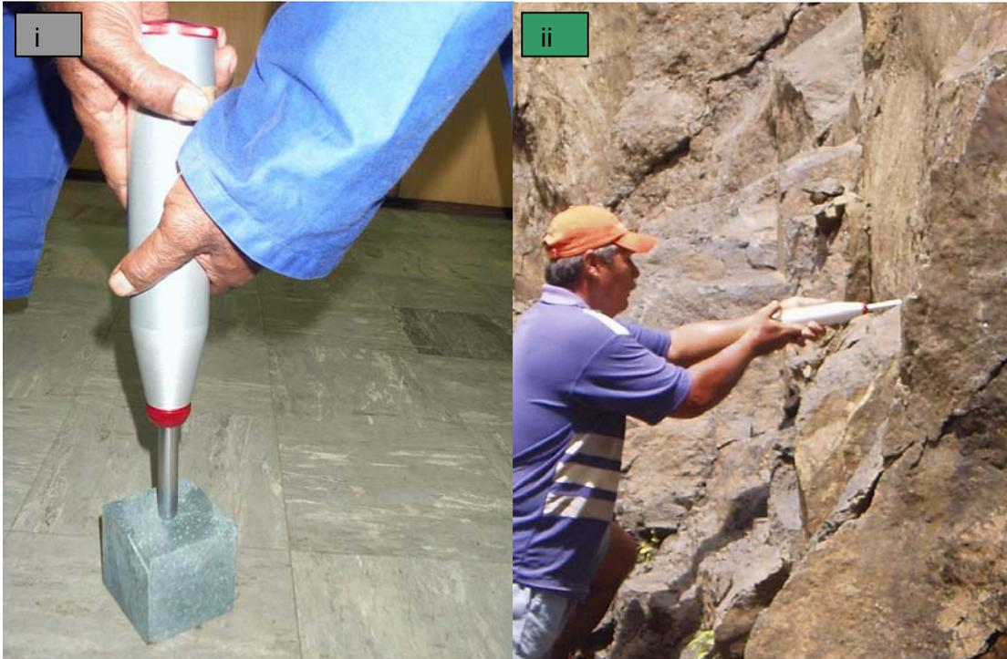
*Figure C. Strength test using a Schmidt Hammer – i) demonstration of how the hammer is being applied on a rock cube; and ii) use of the hammer in a horizontal position against a vertical rock wall.*
